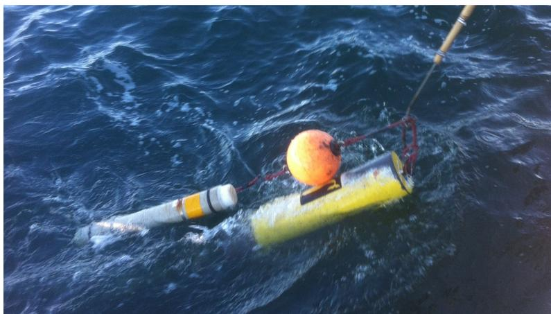
**Figure 3.1:** Photograph showing a recording setup being retrieved. The buoy keeps the setup suspended. The yellow part is the recorder. The gray PVC pipe contains the release mechanism that responds to an acoustic signal containing a password by releasing the setup so that it floats up to the surface.
