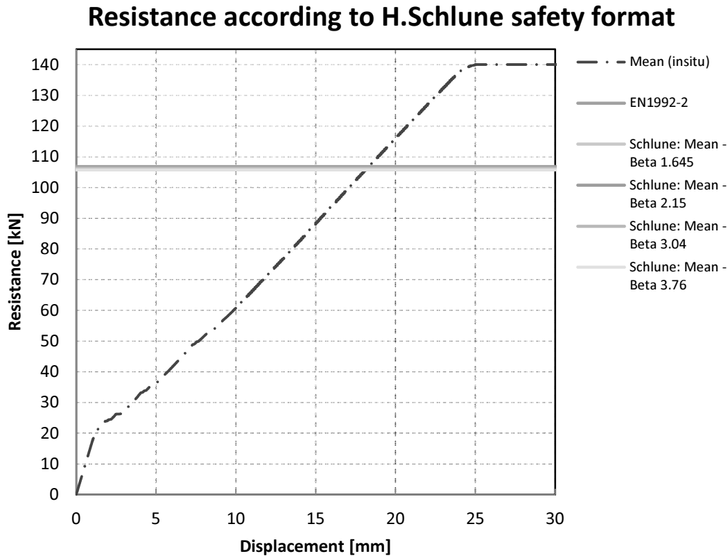
Figure 4.21 The structural resistance according to the proposed safety format by Schlune et al (2010).
