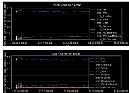
(b) Road condition predictions illustrating both the left (upper) and right (lower) lasers.
