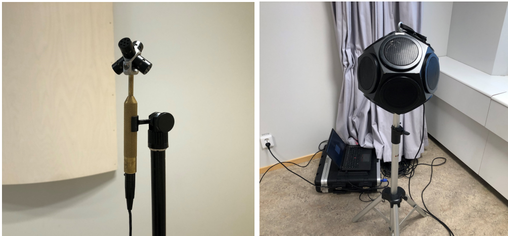
Figure 3.4: Equipment used for measuring room acoustic parameters, Core Sound TetraMic (left) and Dodecahedron omnidirectional speaker (right).
