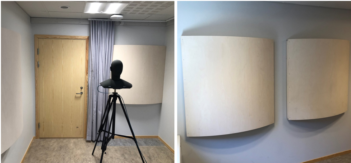
Figure 3.1: The small practice room, binaural recording head Artemis HMS V, and the semi-cylinder diffusers used in the investigation.
