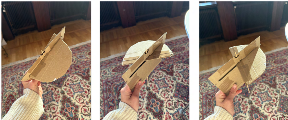
Figure 14: Cardboard mock up used to evaluate a rotational concept principle.
