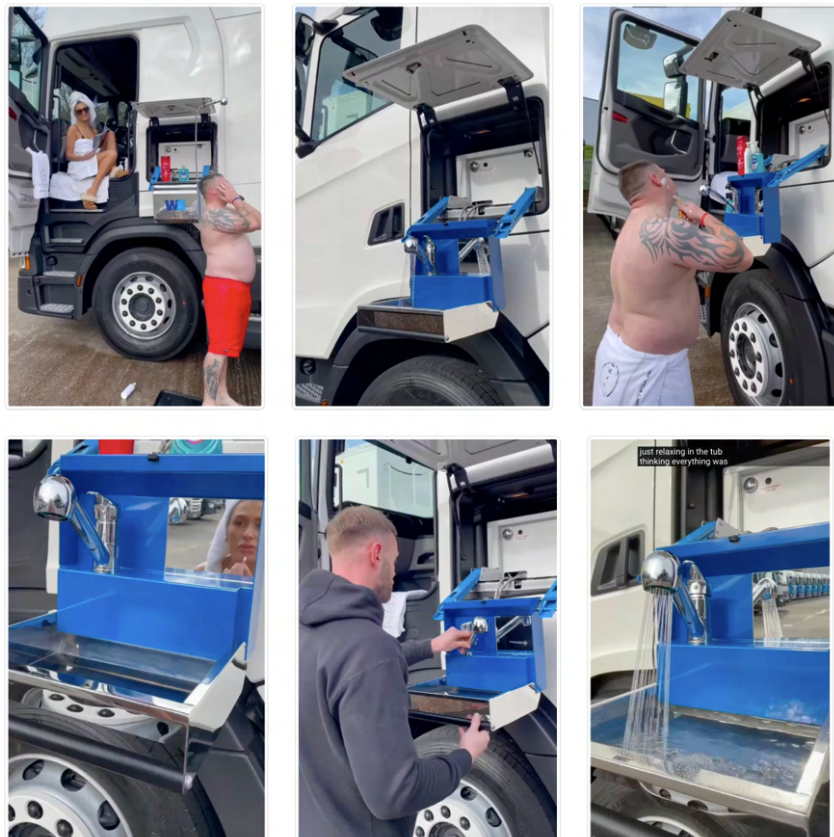
Figure 6: Existing exterior hygiene solution accessible from outside the truck cabin.
