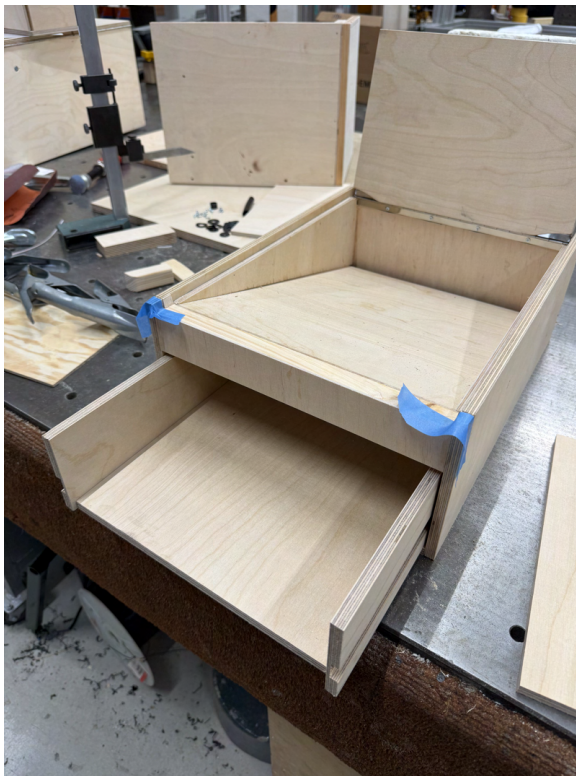
Prototype assembly exploring the pull-out drawer and hinged lid mechanism
