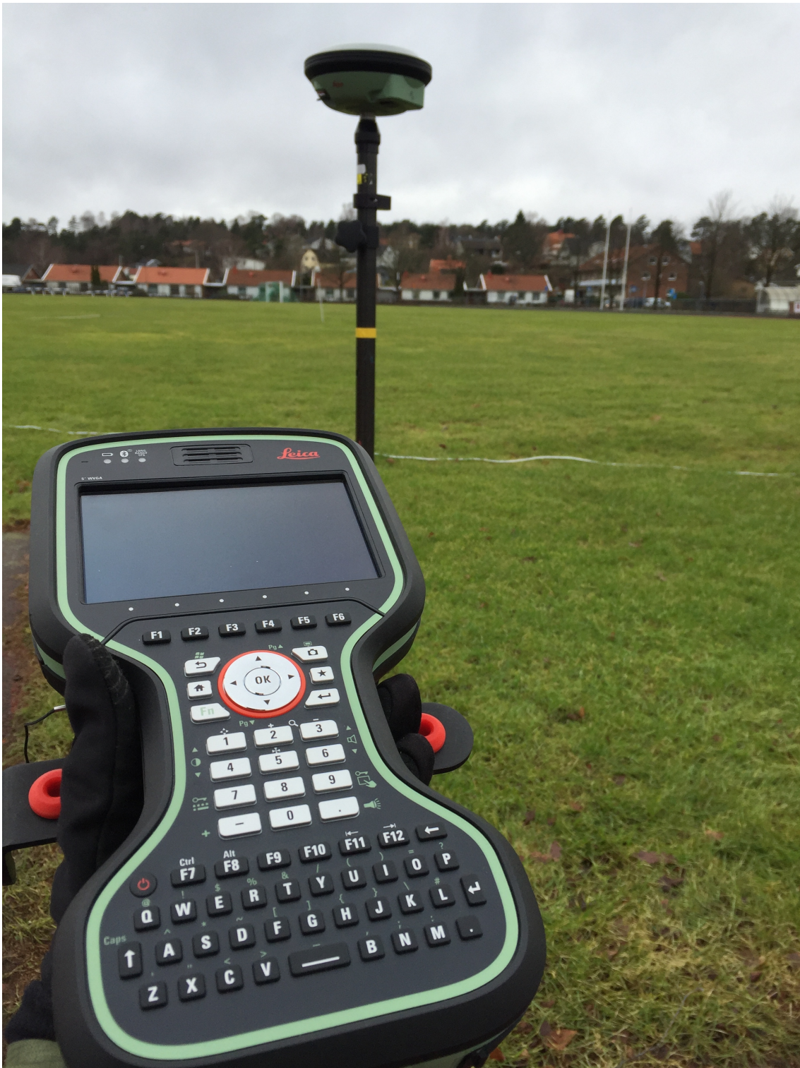
Figure 7: Surveying of positions using Leica GS14 GNSS antenna and a handheld Leica CS20 controller.
