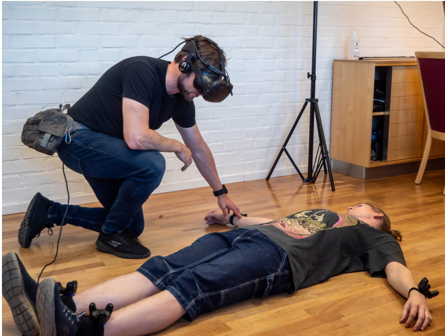
Figure 5.4: A medically trained participant of the first interactive demo tests the simulator using a HMD. A member of the project group acts as the wounded soldier, tracked with Vive Trackers on their wrists and ankles.
