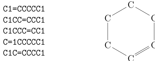
Figure 2.1: Cyclohexene molecule and several valid SMILES encodings. Cyclohexene consists of a closed ring of carbon atoms, denoted by C1 , with a double bond marked by = .
