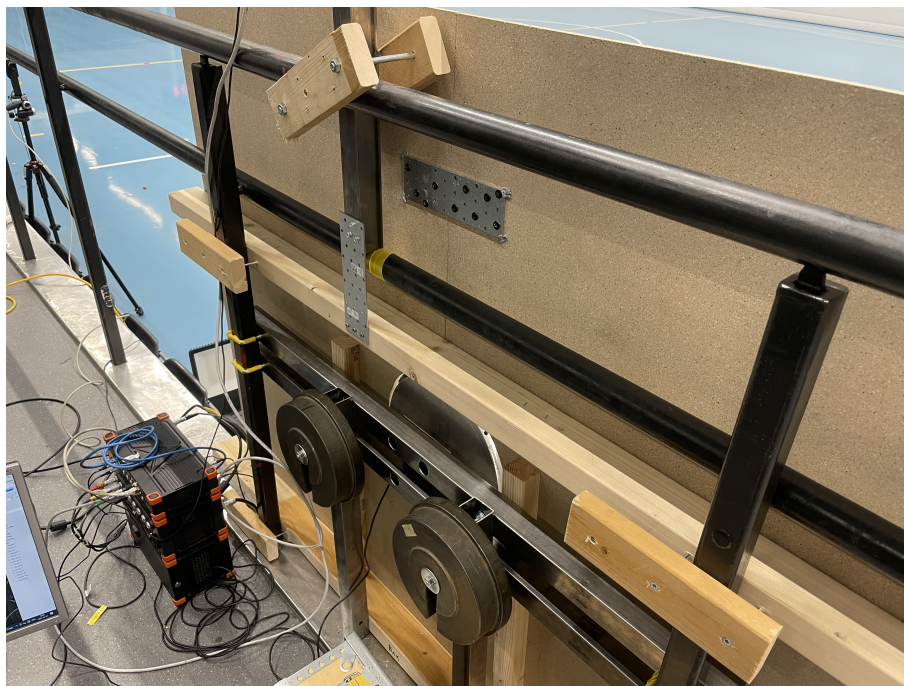
Figure 3.4: Back side of test rig and load cell setup
