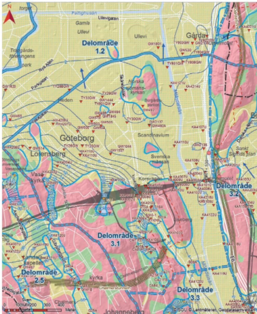
Figure 2.10: Soil map with groundwater head in the lower soil aquifer, pink=rock outcrop, yellow=cohesive soil, green=glacial till (Sundkvist & Wallroth, 2016). Adapted with permission.
