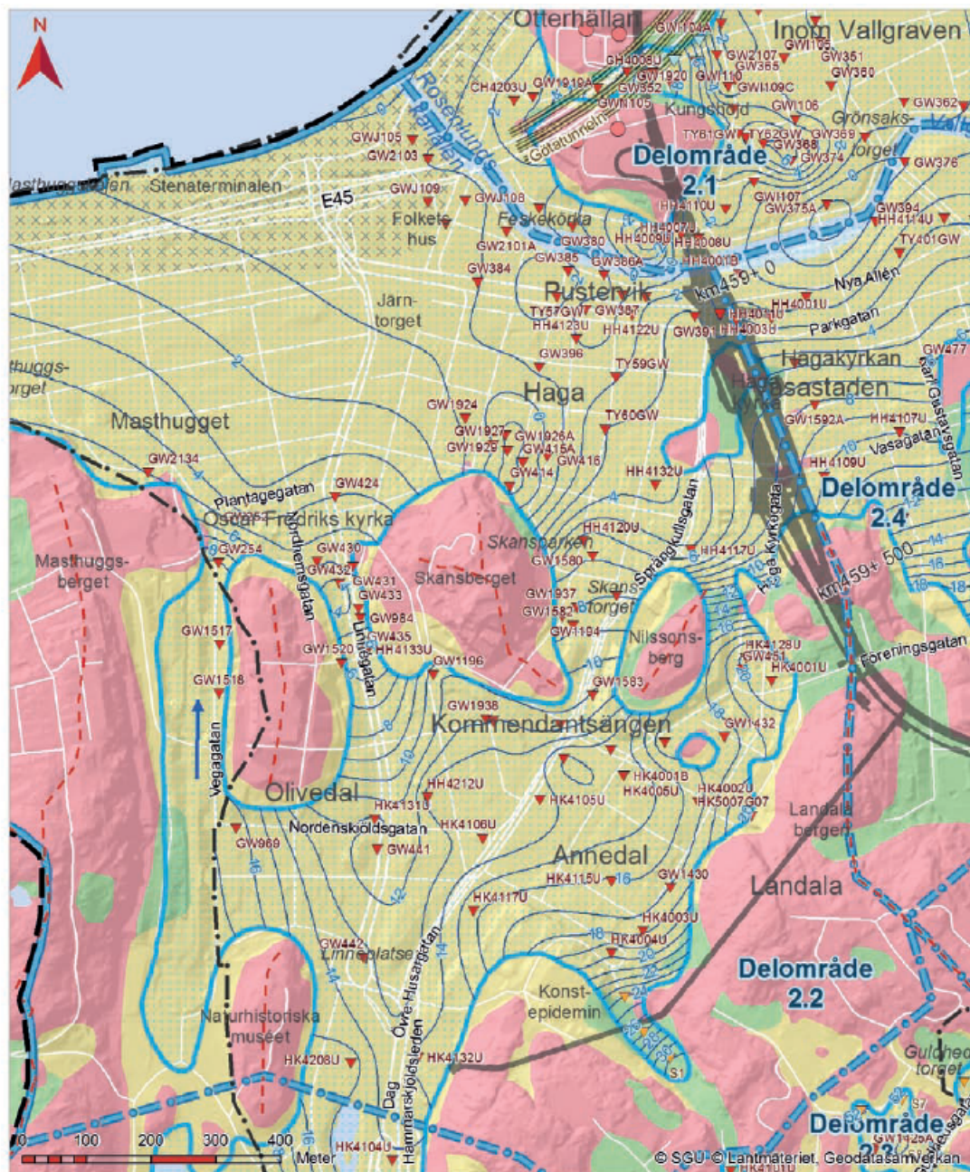
Figure 2.7: Lower soil aquifer. Groundwater head, flow direction and water divides (Sundkvist & Wallroth, 2016).
