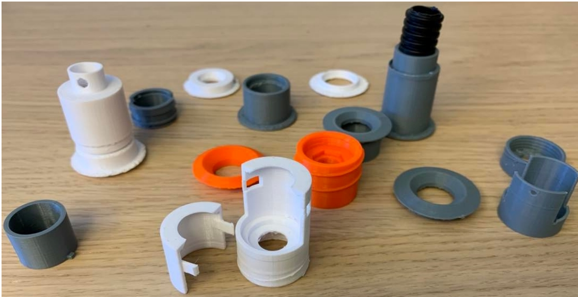
Figure 5.13: Testing different concepts and function with 3D printed parts
