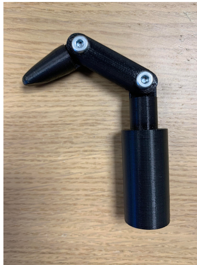
Figure 4.16: Test probe according to IEC 61032
