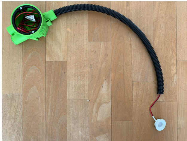
Figure 4.14: Overview of installation of a downlight
