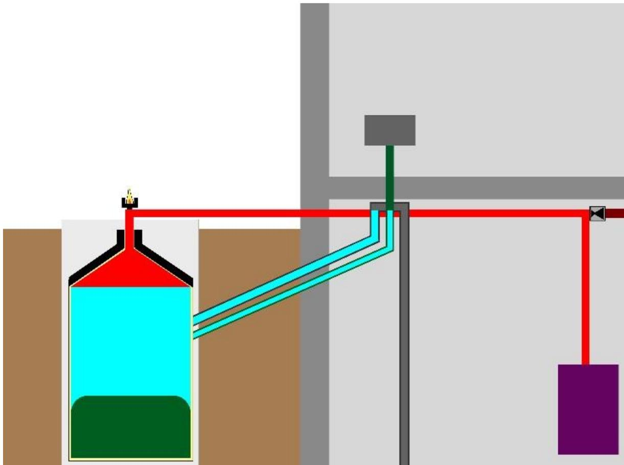
Figure 10 – Concept 4: Well Reactor with Integral Gas Holder
