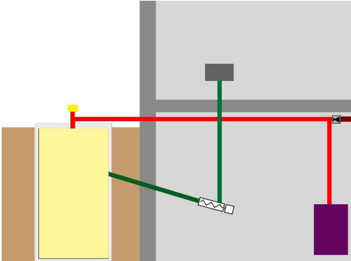
Figure 16 – Concept 10: Well Reactor with Integral Gas Holder and Pump
