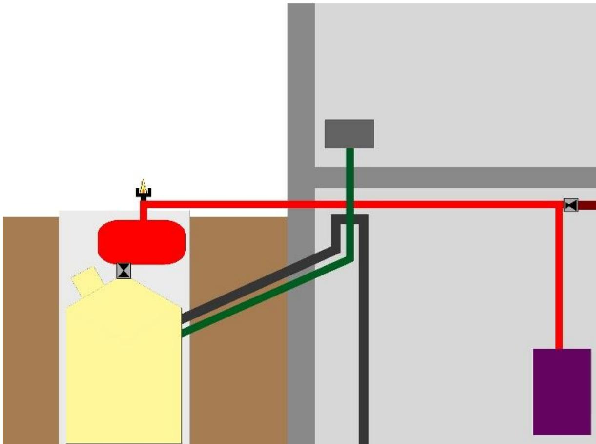
Figure 9 – Concept 3: Well Reactor with Gas Holder
