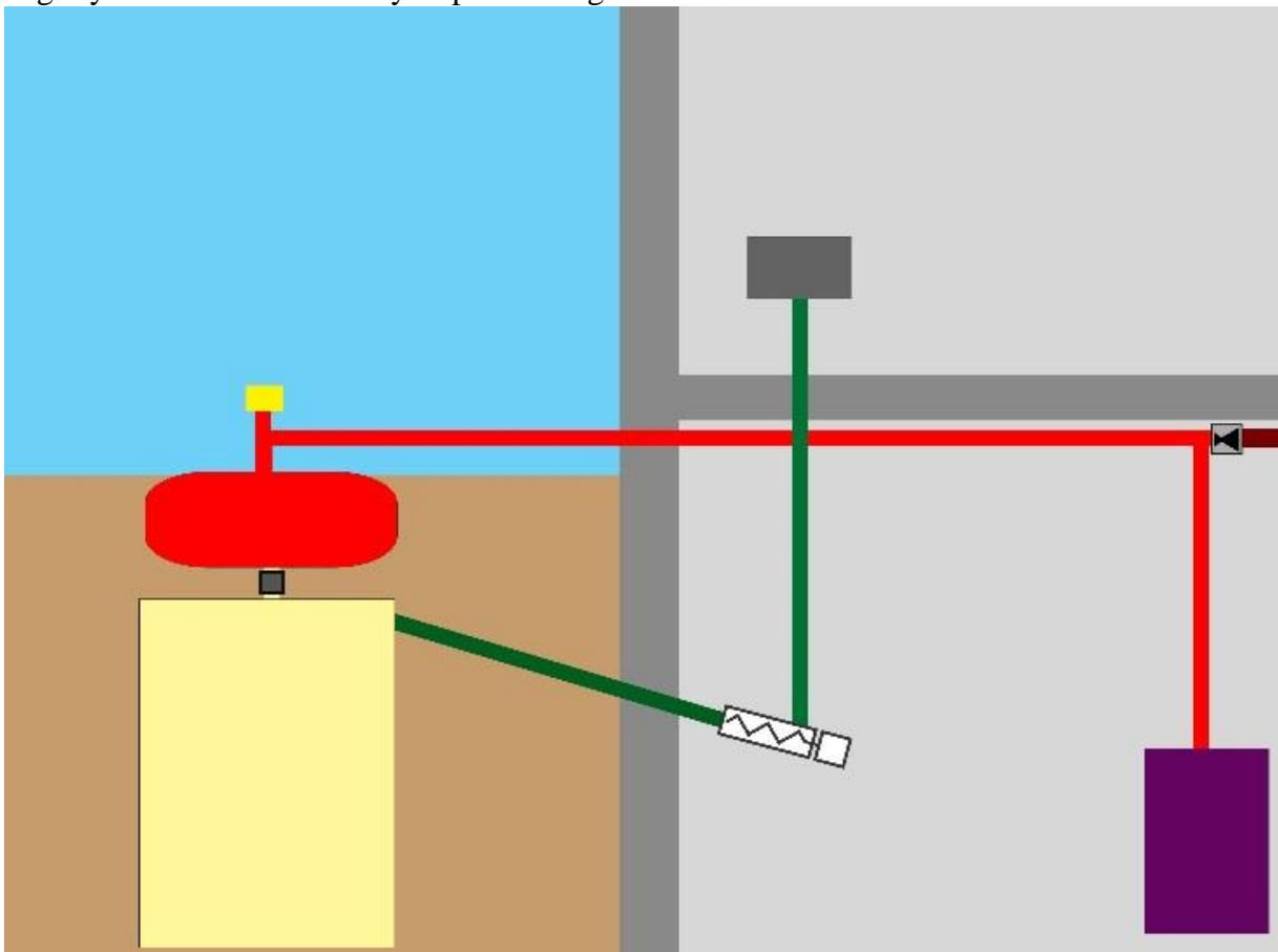
Figure 15 – Concept 9: Well Reactor with Gas Holder and Pump
