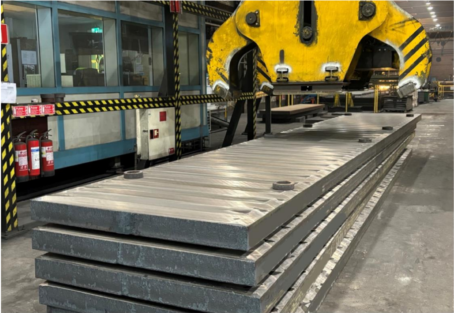
Figure 17: Hot ground slabs ready for cold grinding
