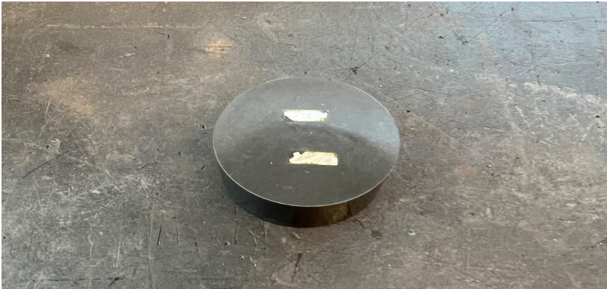
Figure 34: Fully Encapsulated Sample After Hot Pressing, Ready for Further Processing.
