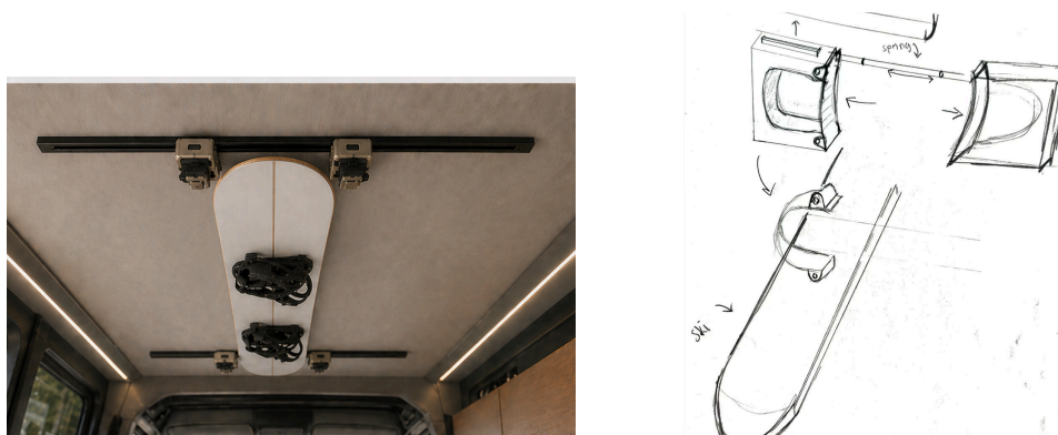
Figure 36. AI-generated interpretation and hand-drawn sketch of gear hooks.
