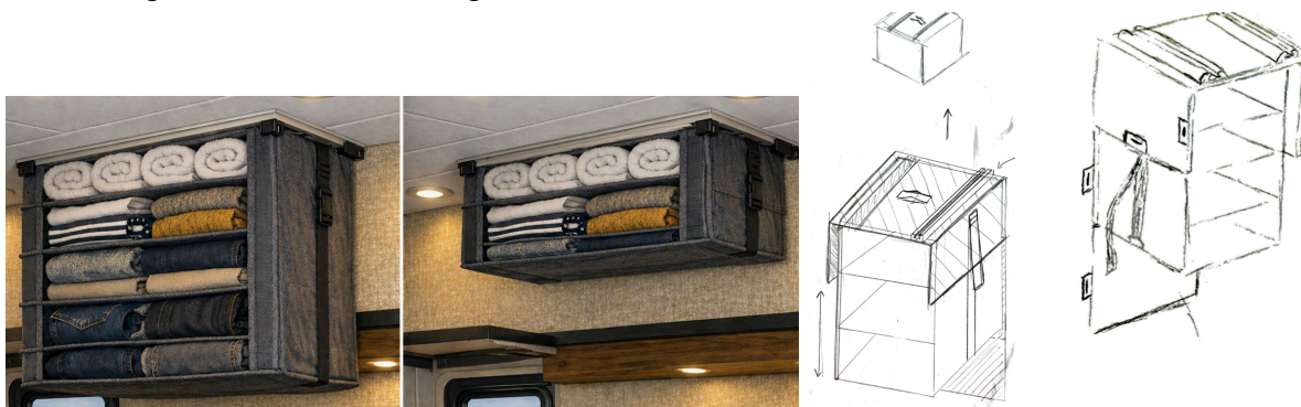
Figure 26. AI-generated interpretation and hand-drawn sketches of compressible storage.
