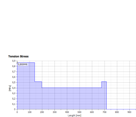
Figure E.13: Tension stress, Autodesk Inventor.
