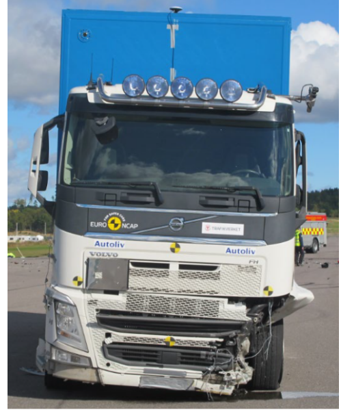
Figure 27: Fractured FUPD after the car-to-HGV crash test, adopted from Thomson et al. (2023).
