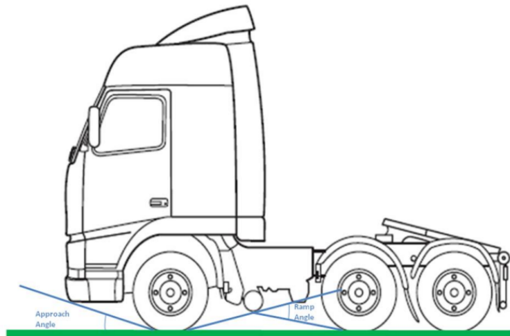
Figure 12: Illustration of approach angle and ramp angle, reproduced from Robinson et al. (2010).
