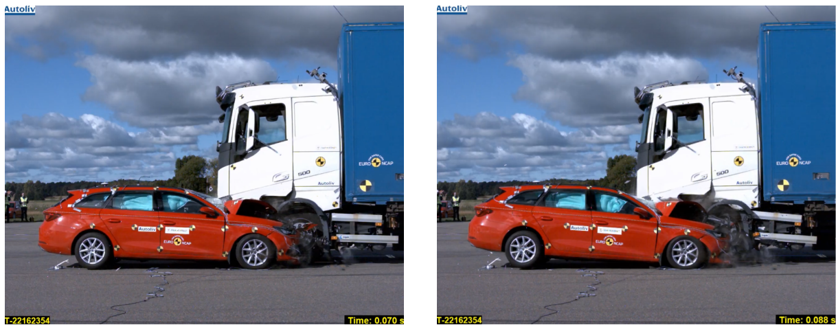
Figure 26: Sequence from the car-to-HGV crash test showing interaction between the PC and the truck front wheel, adapted from Thomson et al. (2023).
