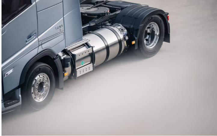
Figure 52: Example of fuel tank placement behind the front axle region, illustrating a possible post-crash vulnerability if the front wheel or axle is displaced rearwards, reproduced from Volvo FH gas-powered , by Volvo Trucks, n.d.
