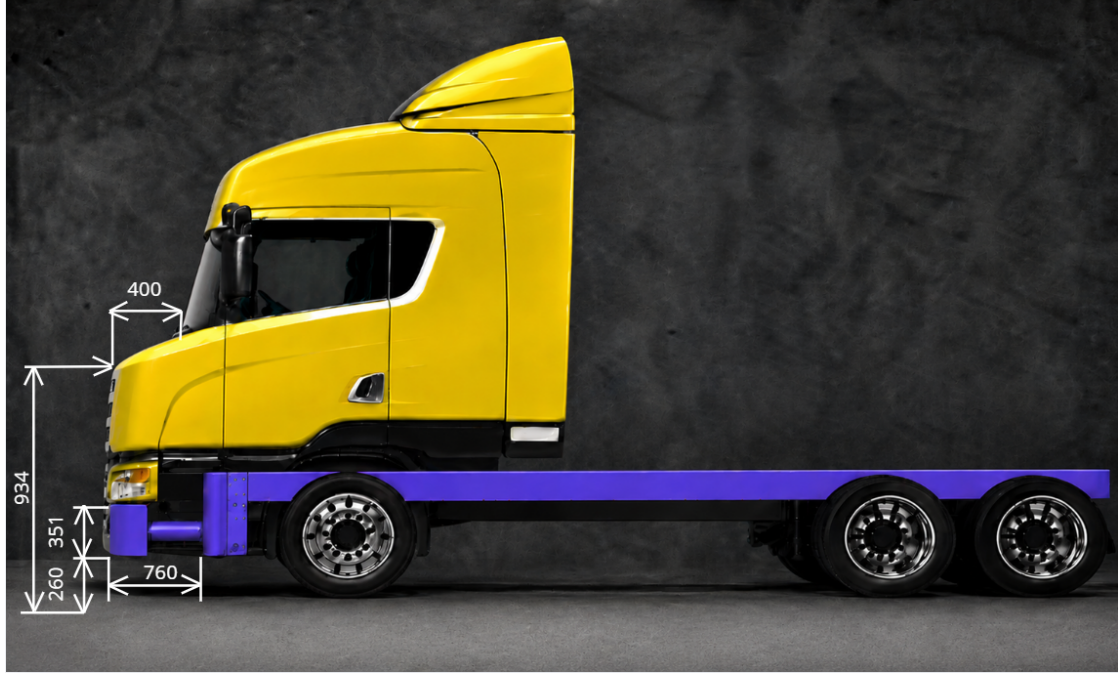
Figure 53: Conceptual extended-front FUP layout, adapted from Danish Transport Authority (2011). Truck shown in the Danish Transport Authority proposal adapted with AI. The original Scania concept used a 600 mm extended front end, while this modified visualization illustrates a 400 mm extended front and the proposed FUP layout used in this thesis. The dimensions are conceptual and not fully scale-accurate.
