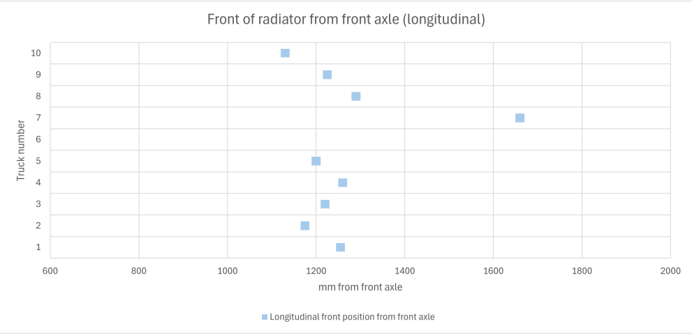
Figure 77: Longitudinal radiator distribution.
