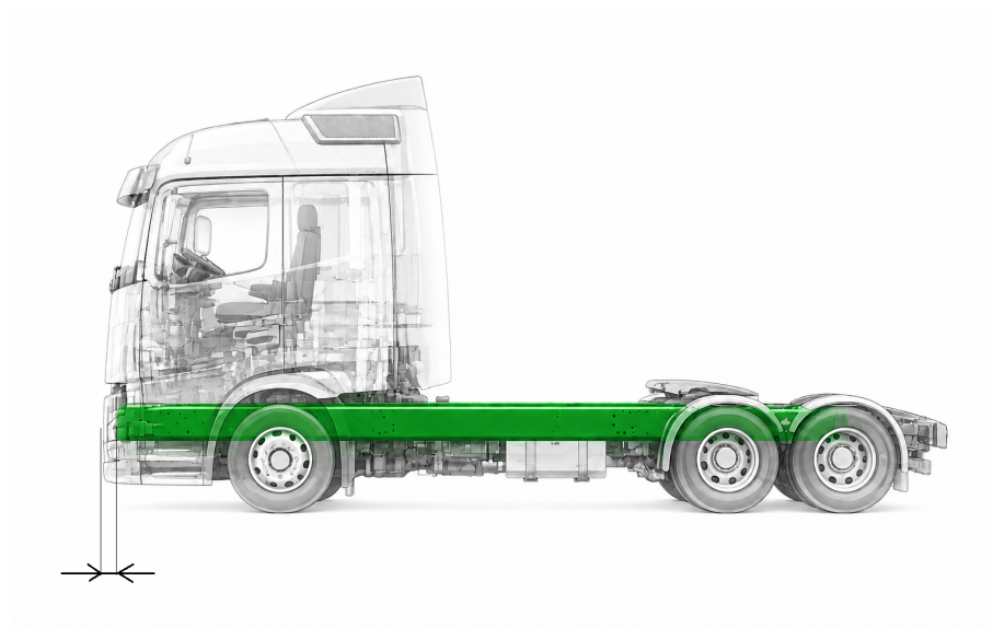
Figure 24: Illustration of frame rail extended close to the front face of the truck generated by AI for visualization purposes.
