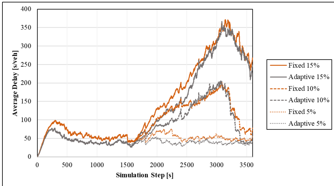
Figure 4.12: Average vehicle delay during sudden demand (steps 1500–2100) at 5%, 10%, and 15% of total demand, across different scenarios
