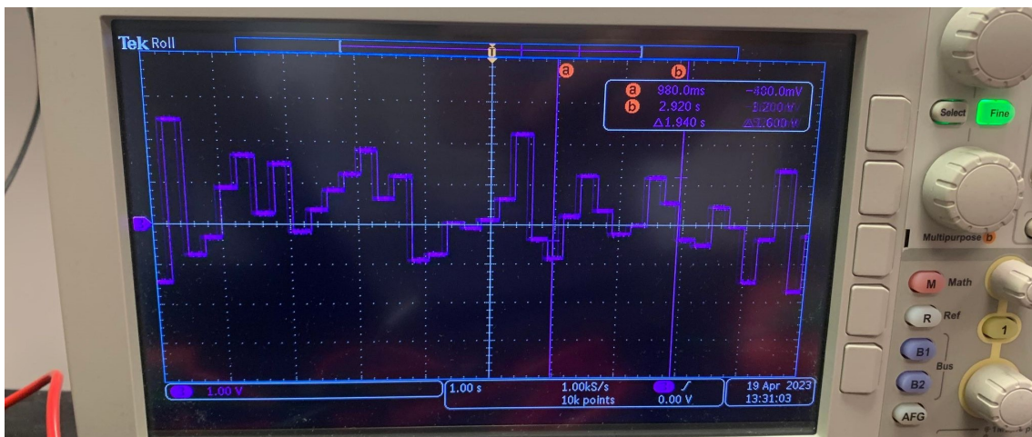
Figure 5.7: The USB2ANY when sending the EMG data to all DAC channels simultaneously. The horizontal axis represents time, where each vertical dotted line marks 1.00 s. The purple plot is the data sent to the ALC through one DAC output channel. Each data point sent to the ALC can be visualized as a level change on the plot, happening approximately every 0.25 s.
