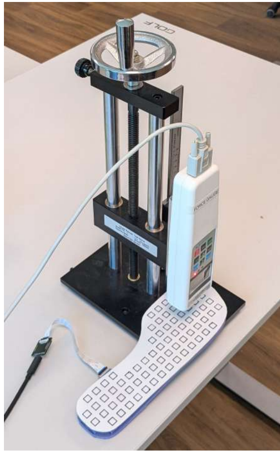
Figure 3.23: Sauter fh-500 test bench with sensor sole.
