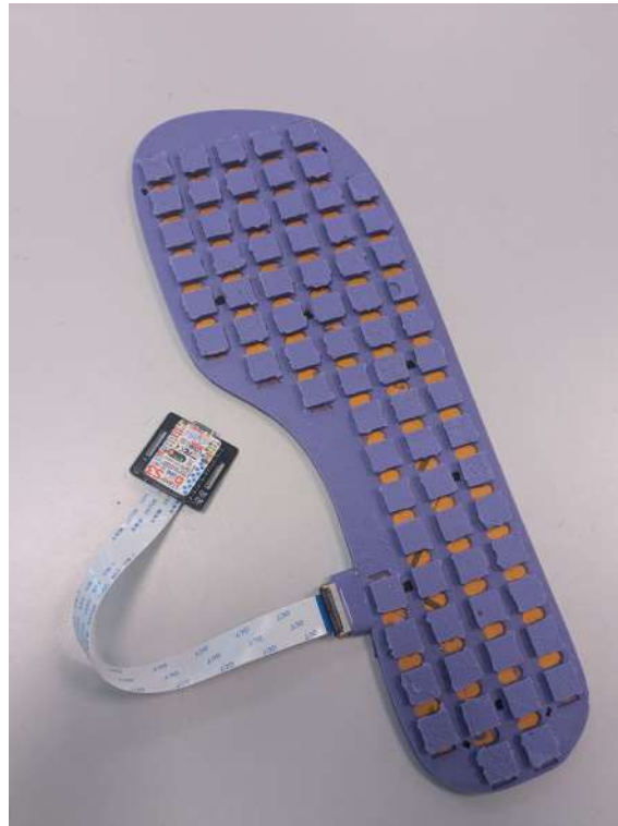
Figure 3.1: Picture of the insole and controller unit.
