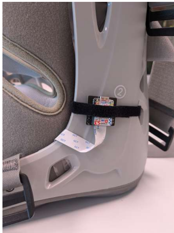
Figure 3.13: Controller unit attached to orthosis.
