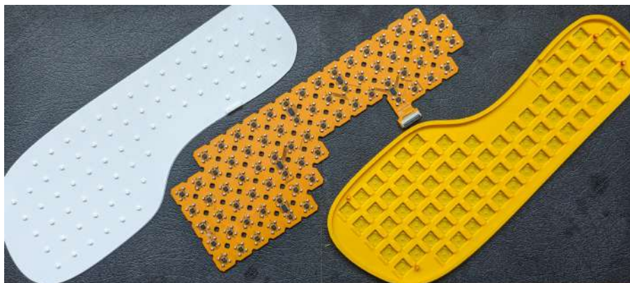
Figure 3.10: Lower half, FPC, and upper half of the first mold.
