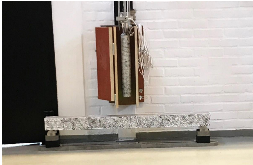
Figure 7.13 Illustration showing test set up for dynamic testing.
