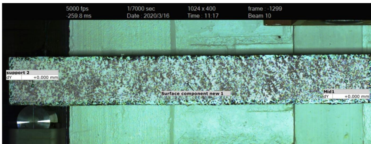
Figure G.1 Image of beam 10-B1-FRP1-D4 before impact, used as reference image.
