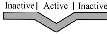
Figure 8.10 Illustration of the active and inactive part of a beam subjected to drop weight impact (Jönsson and Stenseke, 2018).
