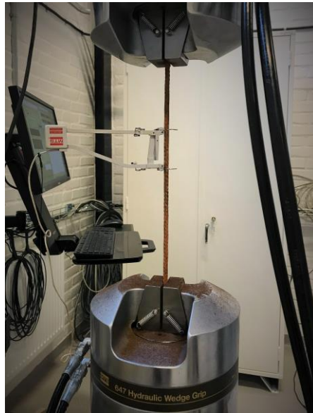
Figure 7.11 Setup for the reinforcement testing in a MTS 380 machine with an extensometer attached to measure strain.
