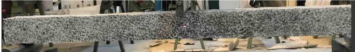
Figure 7.10 Illustration showing the painting pattern for beam 01-B1-FRP0-S.
