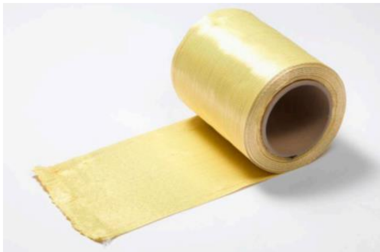
Figure 7.7 S&P A-sheet 120 used in the experiment (from the S&P A-sheet 120 manual).
