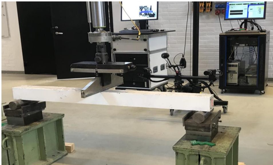
Figure 7.16 Photo of test set up with DIC equipment in the background.
