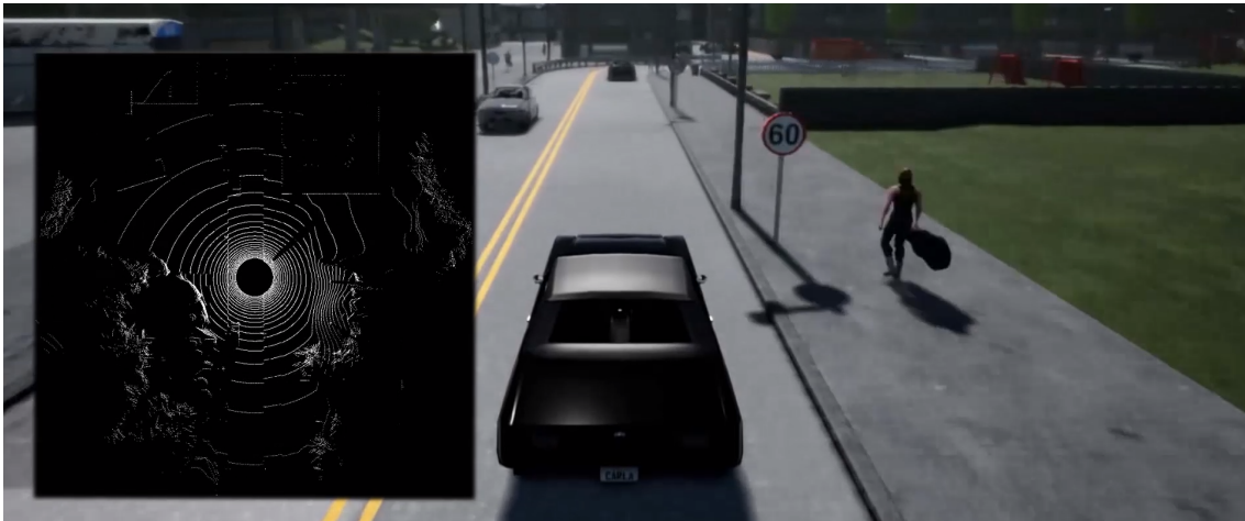
Figure 3.5: Example CARLA simulation scene and corresponding virtual LiDAR output. The overlaid point cloud view shows the LiDAR returns generated from the simulated environment.
