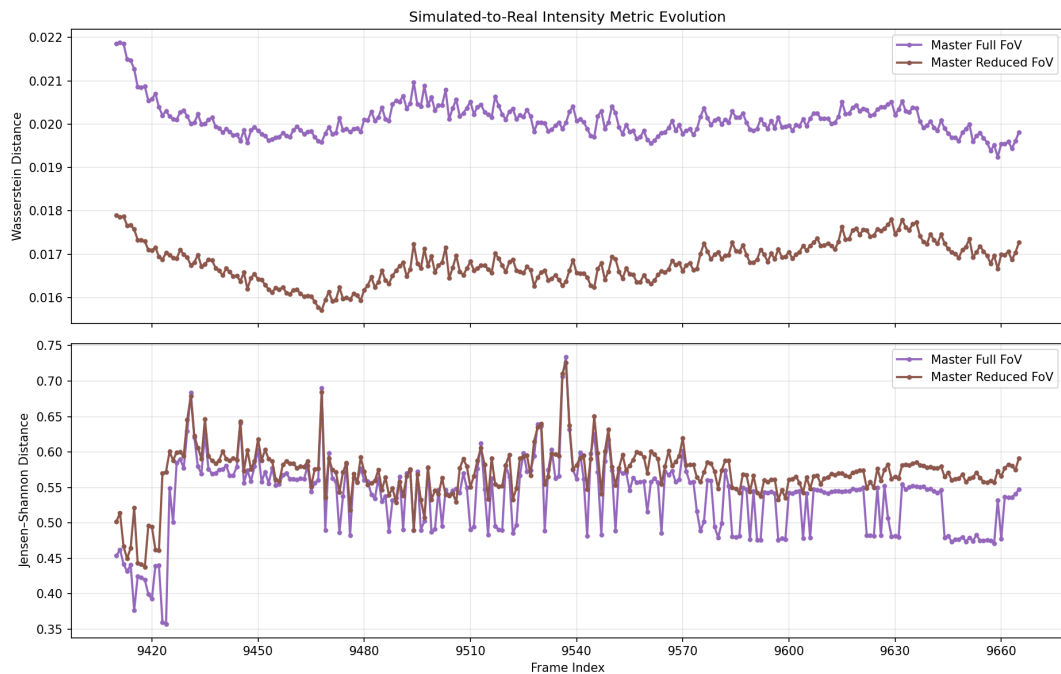
Figure 4.10: Continuous frame-level temporal evolution of the Wasserstein distance (top) and Jensen–Shannon distance (bottom) across the validation Scenario D (Wet) using master fitting curves.
