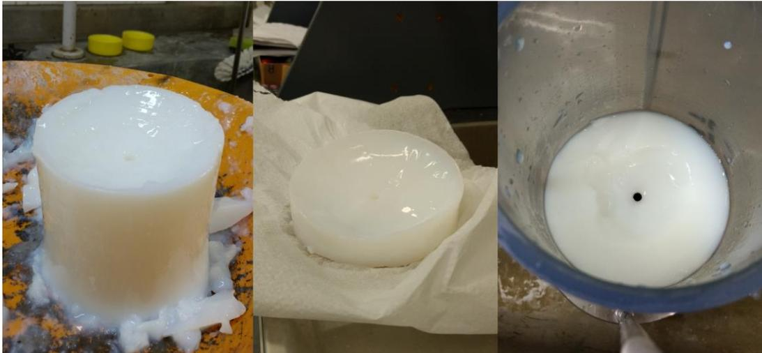
**Figure 12. Half-spherical failure geometry of the silica sol at gel time**
