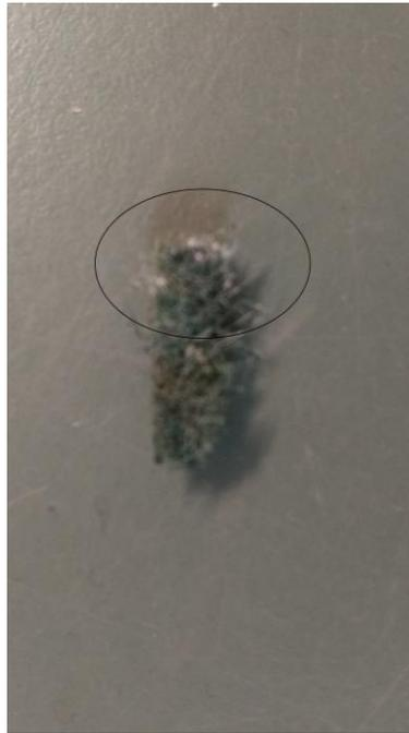
**Figure 14. Dark textile used to clean the inside of the plastic pipes. Remains of silica sol was detected.**
