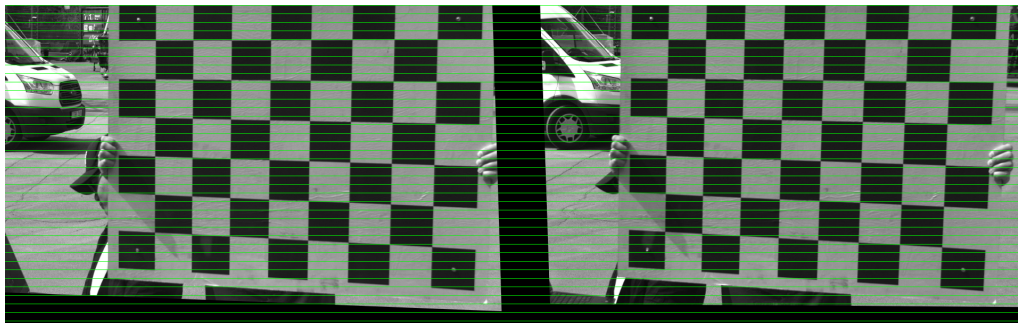
Figure 4.3: Stereo rectification process. Green lines can be viewed as the epipolar lines described in Section 2.1.3.1.
