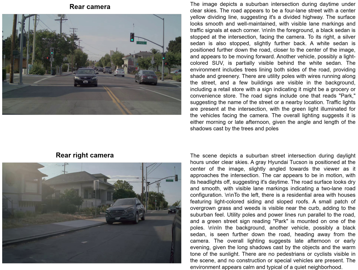
Figure 4.4: Example of multi-view driving scenes together with their automatically generated captions produced by Qwen 2.5 VL 7B instruct model. The figure shows two surrounding camera perspectives: rear camera view, and rear right camera view.
