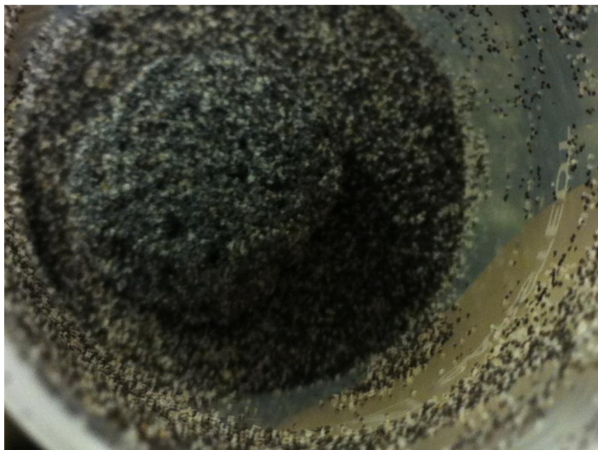
Figure 16 The material, Particles type 1, after the reaction process. Agglomeration of the particles is observed.
