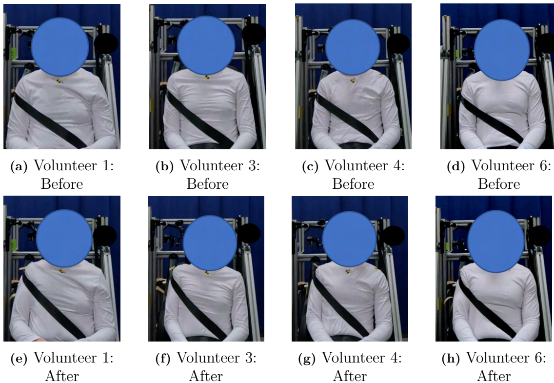
Figure E.1: Images displaying the before and after for 4 out of the 25 volunteers the belt did not reposition for. The shoulder belt position when positioned 10 cm down the arm, before, and the position after the pre-pretensioner was activated in the belt-in-seat installation. The before images are depicted in the top row while the corresponding after images are depicted in the bottom row. The after image depicts when the belt pre-pretensioner held the belt with a constant force in an improper position for the volunteers.
