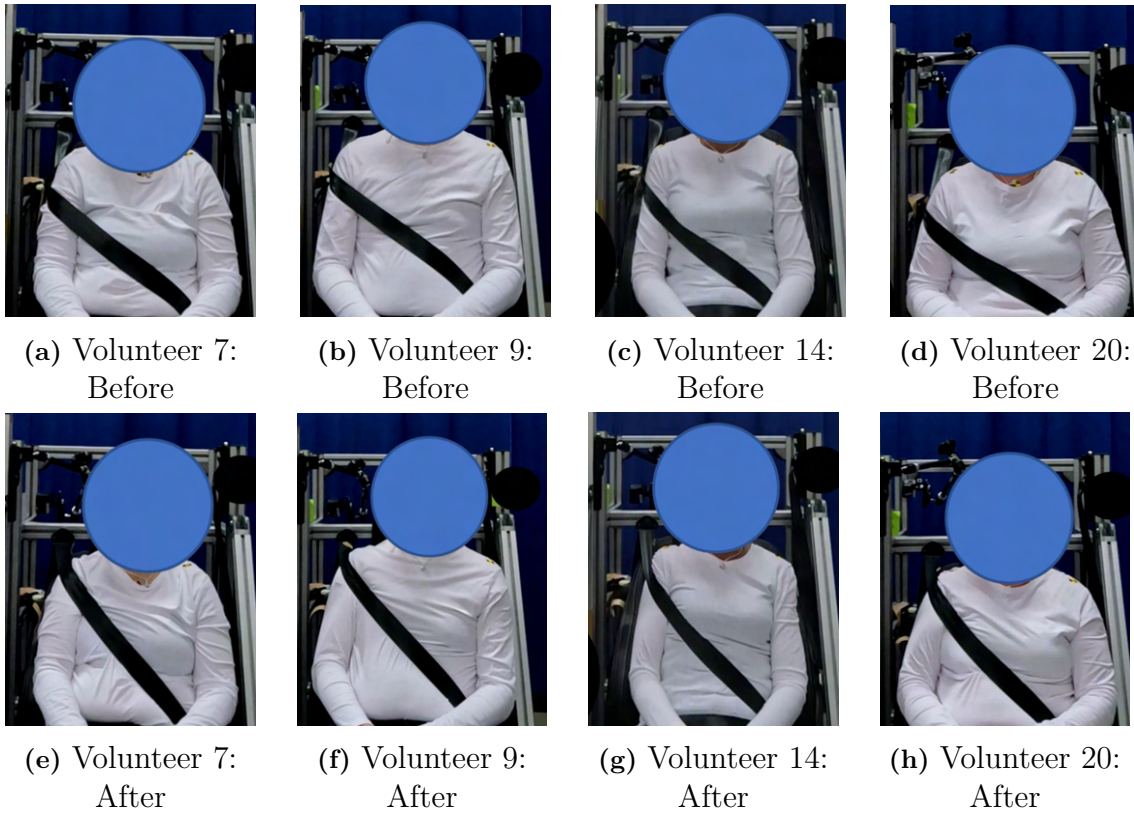
Figure E.2: Images displaying the before and after for 4 out of the 25 volunteers the belt did not reposition for. The shoulder belt position when positioned 10 cm down the arm, before, and the position after the pre-tensioner was activated in the belt-in-seat installation. The before images are depicted in the top row while the corresponding after images are depicted in the bottom row. The after image depicts when the belt pre-tensioner held the belt with a constant force in an improper position for the volunteers.
