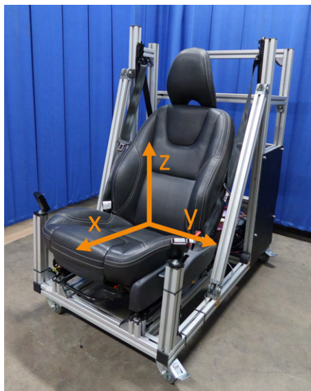
Figure 2.1: The test rig and the coordinate system, with the origin in one H-point.
