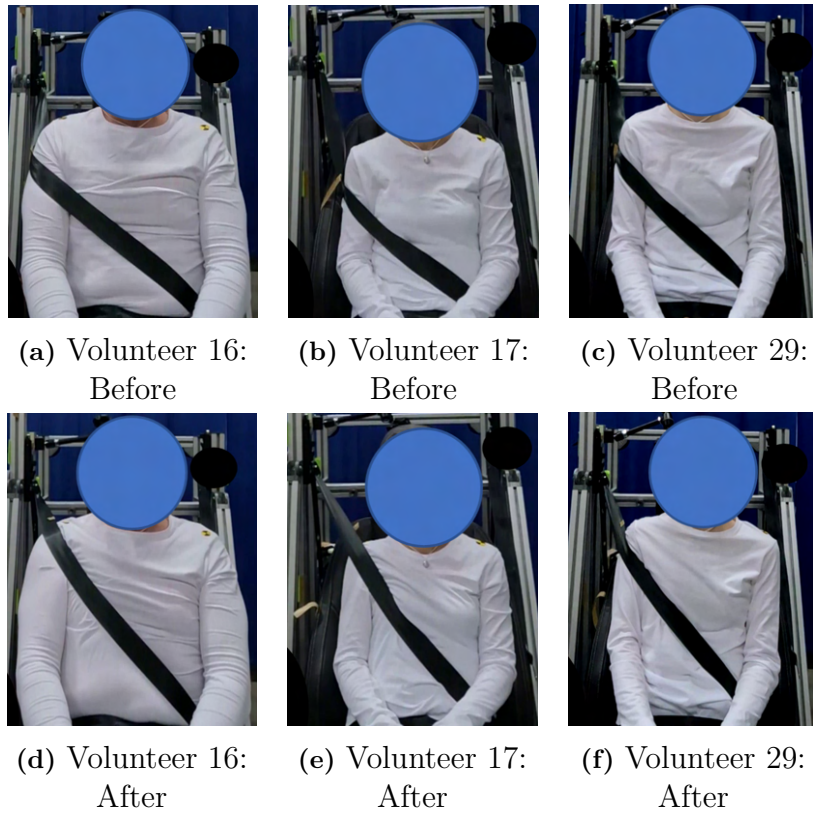
Figure D.2: Images displaying the before and after for the remaining 3 out of the 7 volunteers the belt did not reposition for. The shoulder belt position when positioned 10 cm down the arm, before, and the position after the pre-pretensioner was activated for the most forward position in the test rig. The before images are depicted in the top row while the corresponding after images are depicted in the bottom row. The after image depicts when the belt pre-pretensioner held the belt with a constant force in an improper position for the volunteers.
