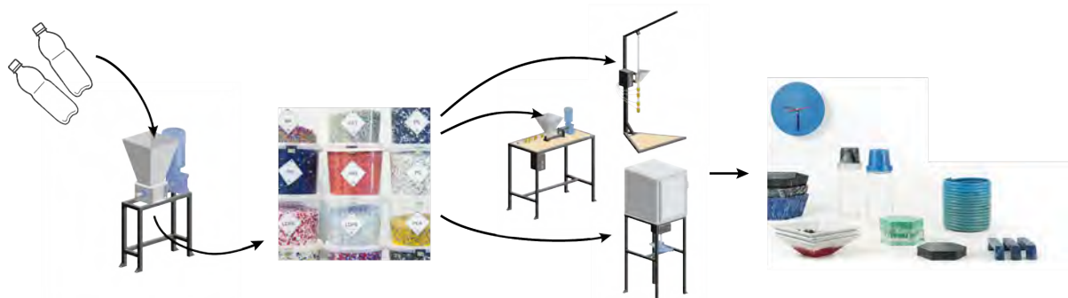
Figure 6. Precious Plastic proposes a process where clean, dry and sorted plastic is collected. The shredding machine resizes the plastic waste to granules. The granules are then manufactured through one of the three creating machines to new products. Reprinted with permission.
