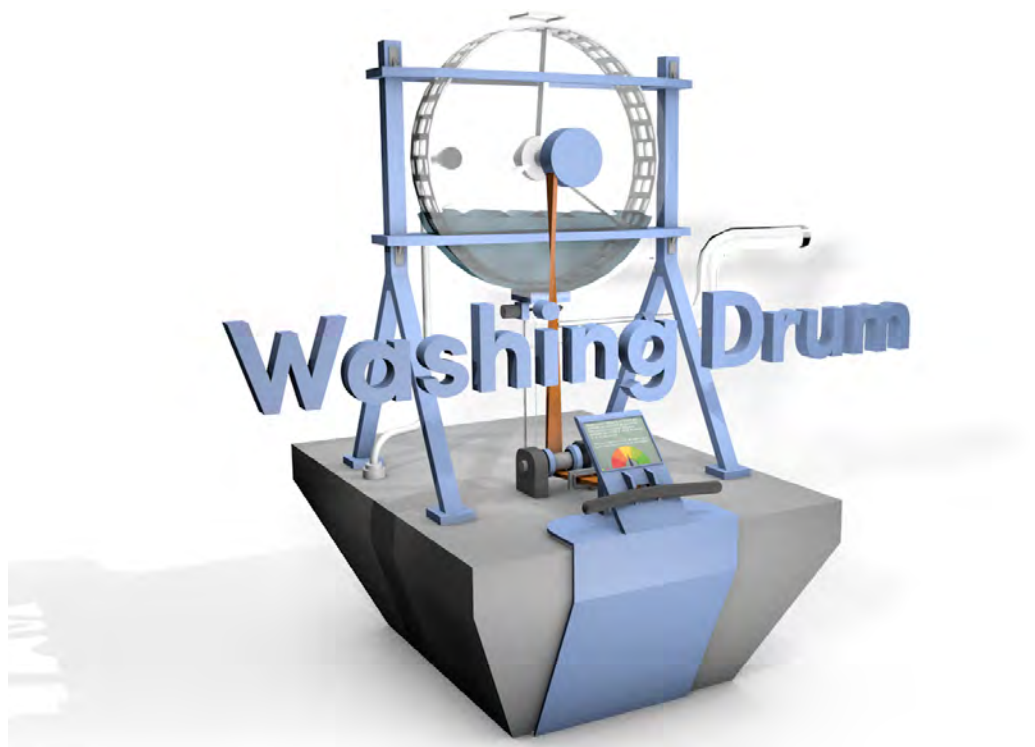
Figure 44. The Washing Drum. This element's main task is to clean the plastic granules from residues and impurities.
