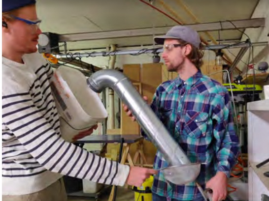
Figure 13. Testing the feasibility of transporting wet granules using high pressure air.
