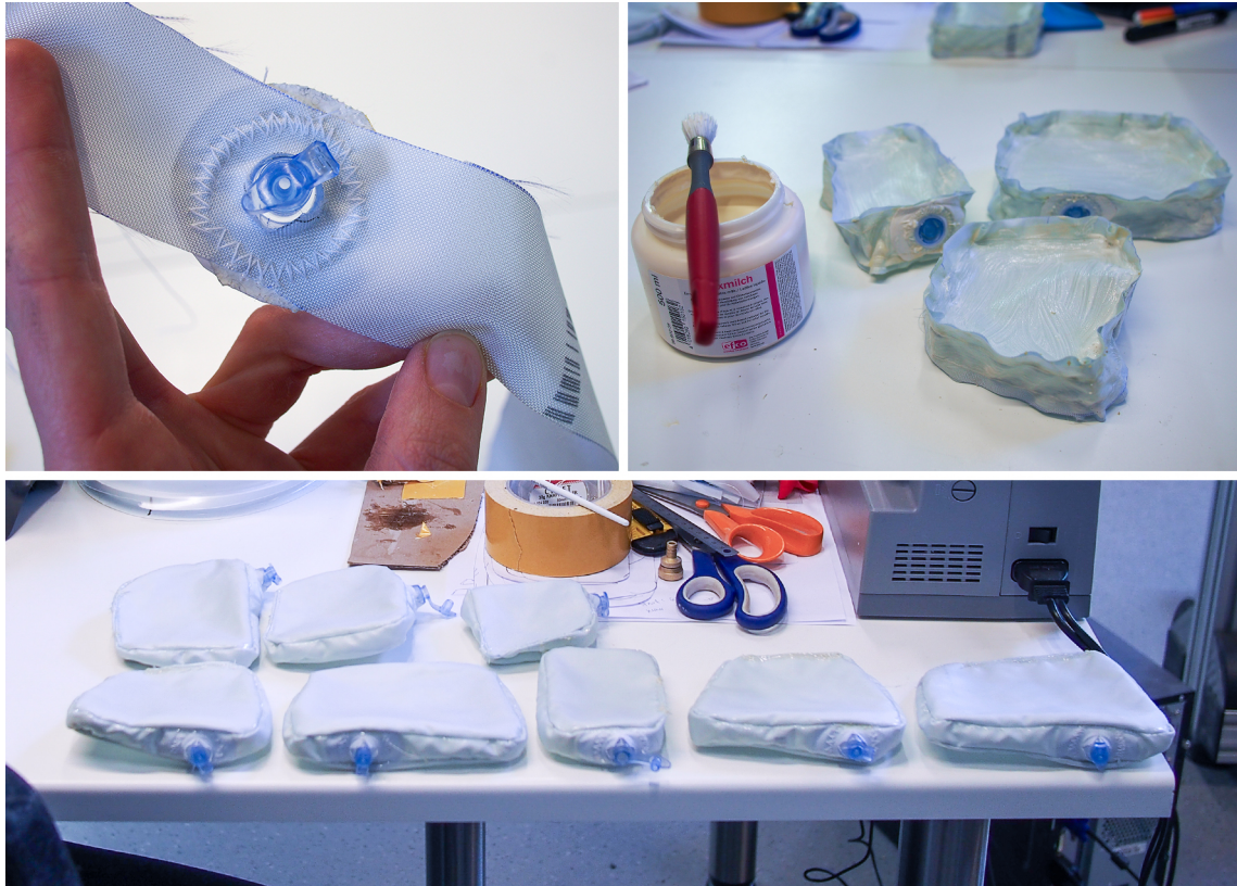
Figure 7.4: The prototyping process from attaching valves to sealing the seams with latex, to the finished airbags
