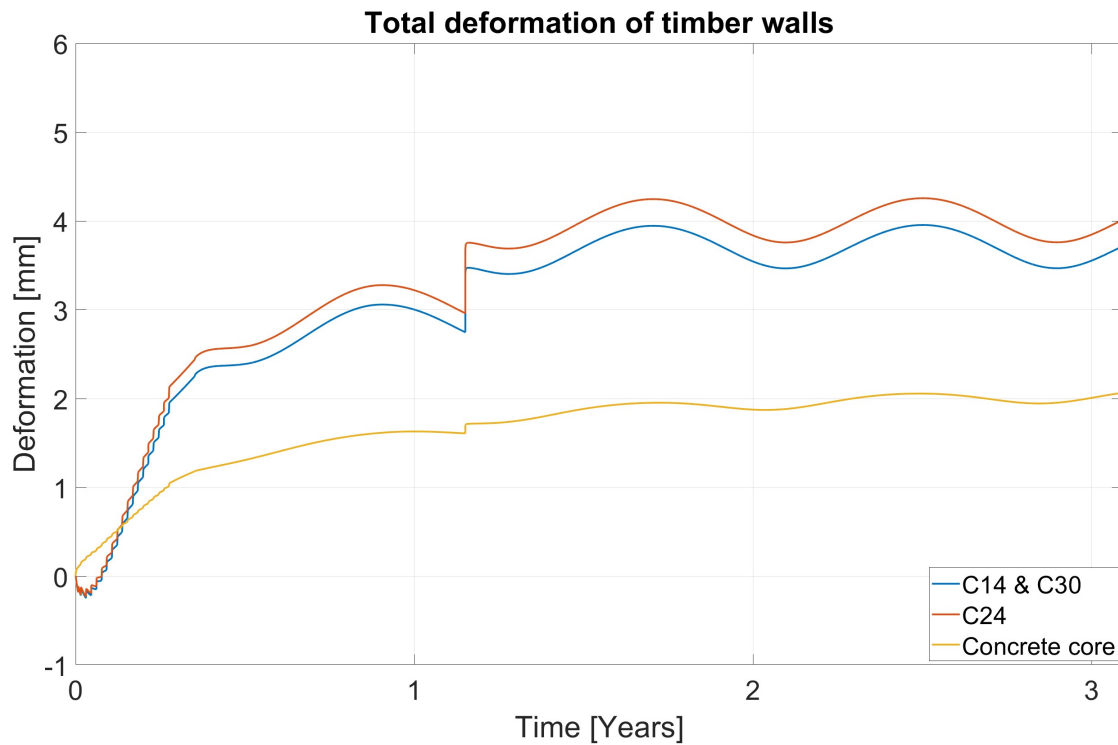
Figure 6.8: Vertical deformations of timber wall element for scenario: varying strength class of timber. Concrete core element deformation is shown as a reference.
