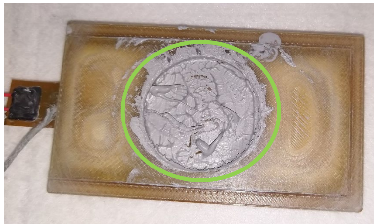
Figure 19: Improper application of thermal paste
