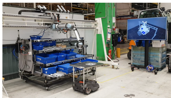
Figure 1.1: Collaborative bin picking by an industrial robot[7]. Redistributed with permission.
