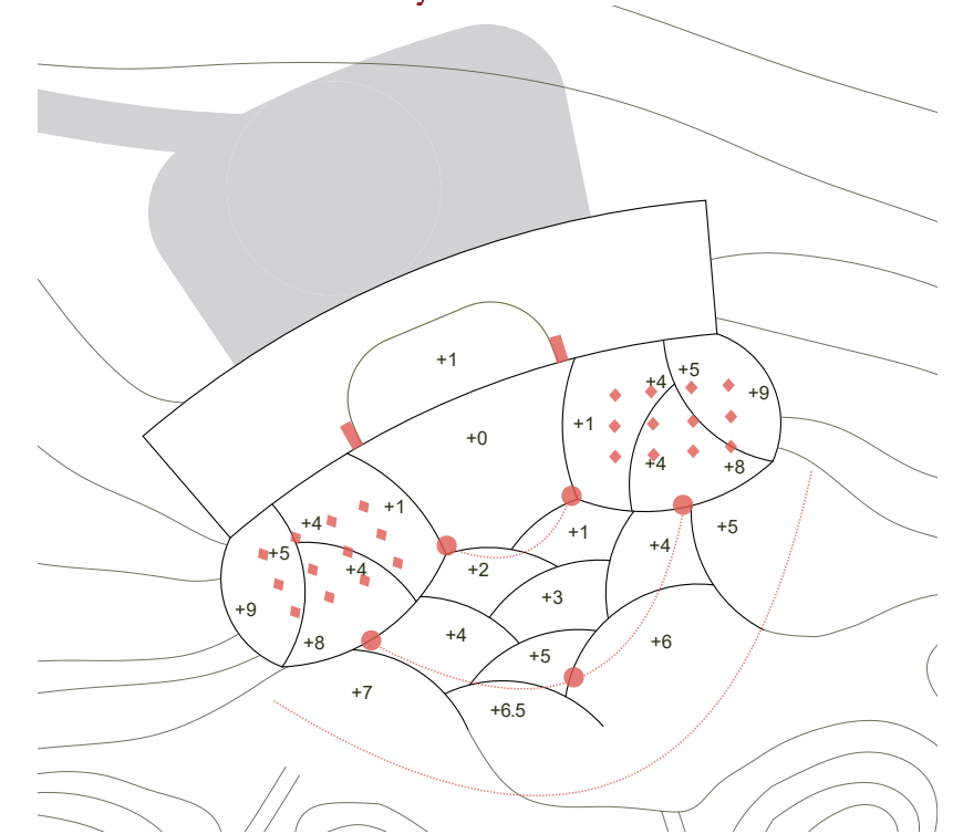
Cross firing clusters (front zone), overhead distribution grid (seated zones), and line array positions (middle and back zones)
