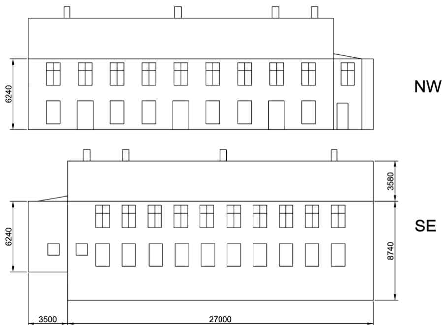
Figure 6.3 Sketches of the long facades. Top figure: Northwest façade, bottom figure: southeast façade [mm].
