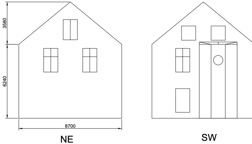
Figure 6.4 Sketches of the short sides. Left figure: Northeast facade, right figure: southwest façade [mm].
