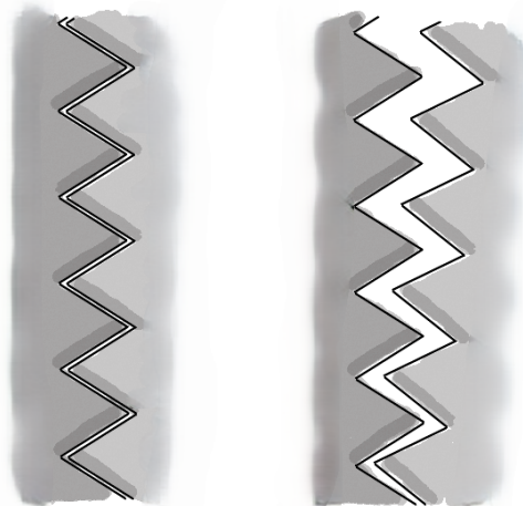
Figure 27: Threads separating as a result of uneven clamping
