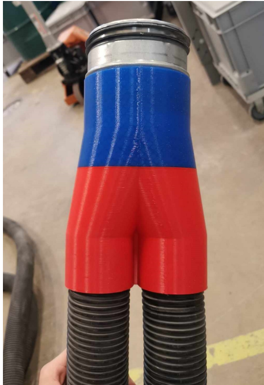
Figure 5.2: Y-cross connection for the connection of two vacuums onto the outlet of the rig.
