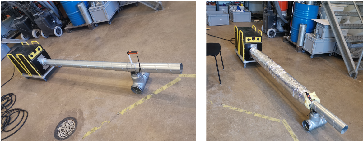
Figure 3.1: Insulation test setup, duct pipe without insulation to the left and duct pipe with insulation to the right.
