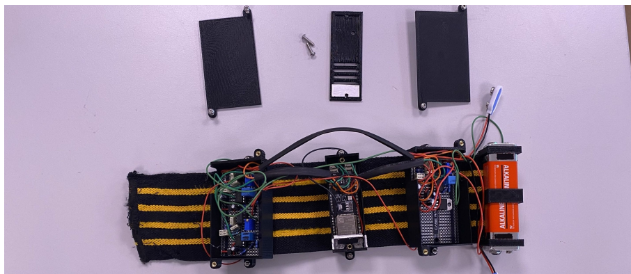
(c) Outwards-facing side of the sEMG band with open circuits, rolled out
