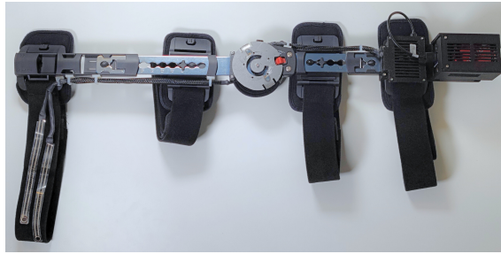
Figure 5.20: The orthosis without the motor and motor housing being fully extended.
