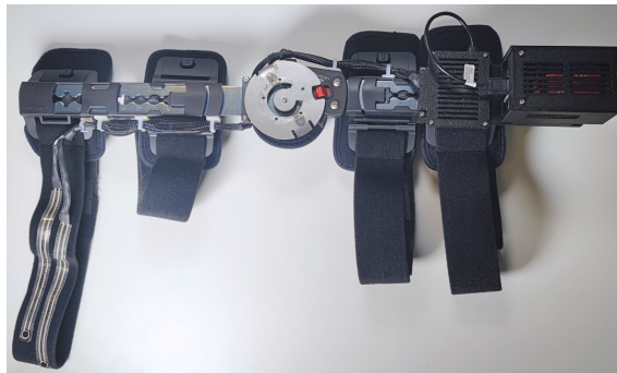
Figure 5.21: The orthosis without the motor and motor housing being fully retracted.
