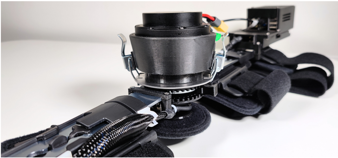
Figure 5.18: Close up of the final assembly showing the two eccentric locks on the side of the motor housing connecting to the attachment plate.
