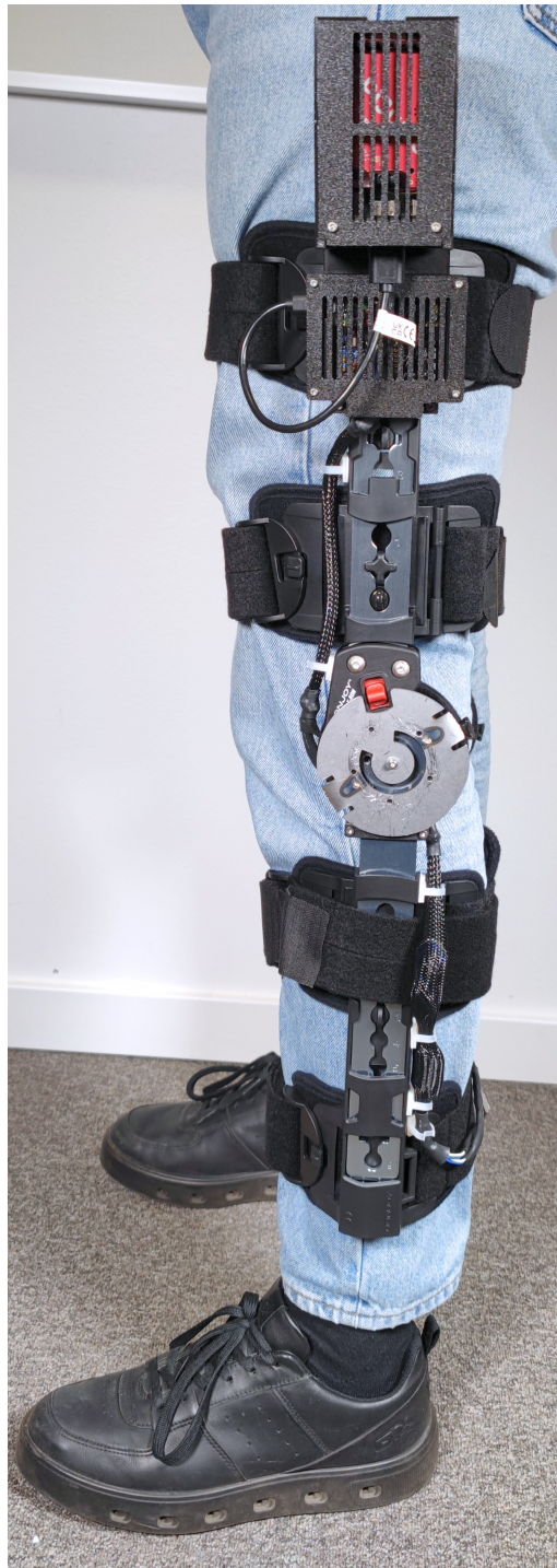
Figure 5.27: The orthosis without the motor worn by a user, showing how the construction fits and aligns with the leg.
