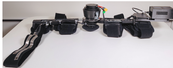
Figure 5.25: Side view of the full assembly with all components (motor, motor housing, attachment plate, angle limiters, electronics housing, encoder housing, force sensors and cables).
