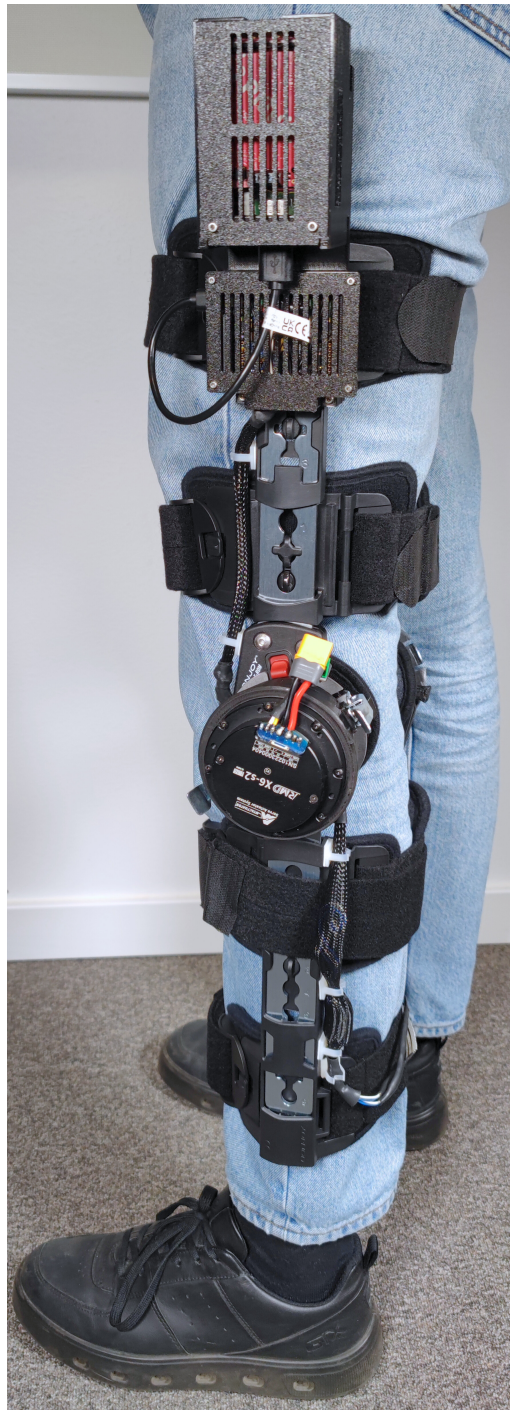
Figure 5.28: The orthosis fully assembled worn by a user, showing how the construction fits and aligns with the leg.
