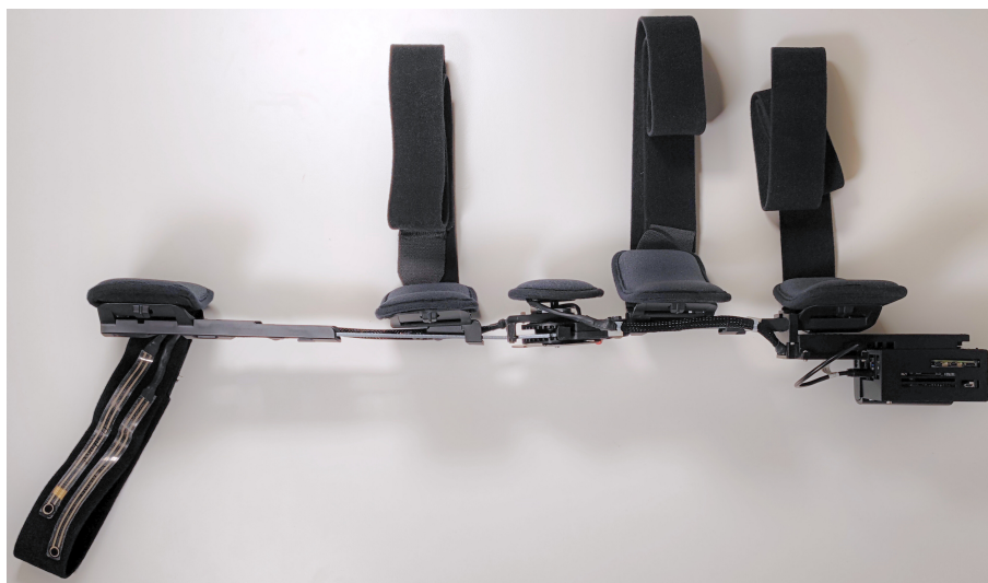
Figure 5.26: Side view of assembly without the motor and motor housing, and only the attachment plate, angle limiters, electronics housing, encoder housing, force sensors and cables.
