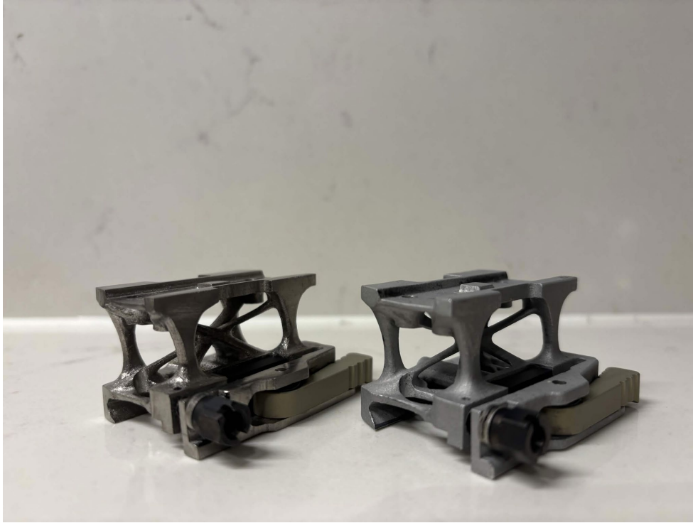
Figure 16: Isometric view of real life assembled mounts, left titanium, right aluminum.
