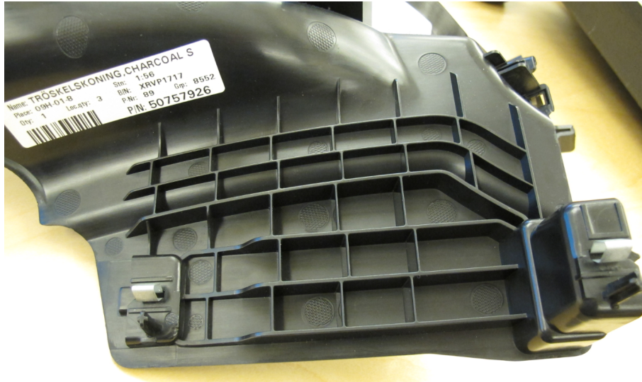
Figure 6: Rib structure underneath the rear door sill mould.
