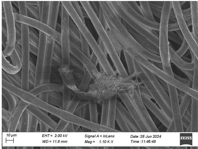
Figure 4.21: Sintered F-H23 in which PTFE particles can be seen adhered around the fibers at 1.10Kx magnification.
