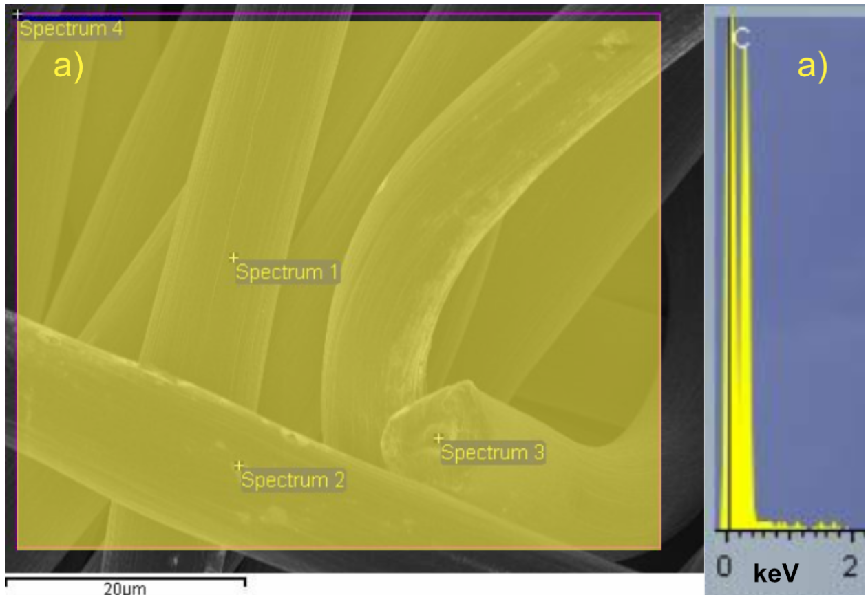
Figure 4.24: EDX analysis of plain F-H23.
