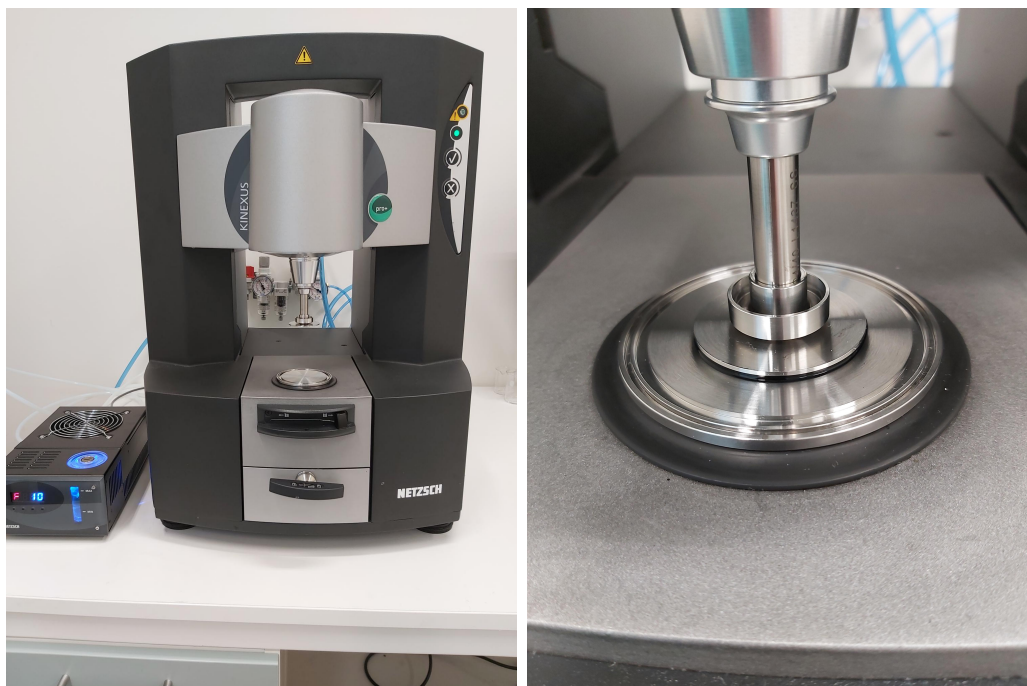
Figure 3.6: Kinexus rotational rheometer fitted with C/P 4/40 with a solvent trap in loading position (left) and close up of set up in loaded position with catalytic ink sample (right). During measuring, the geometry and sample are covered with a hood to minimize evaporation and protect from splashing.
