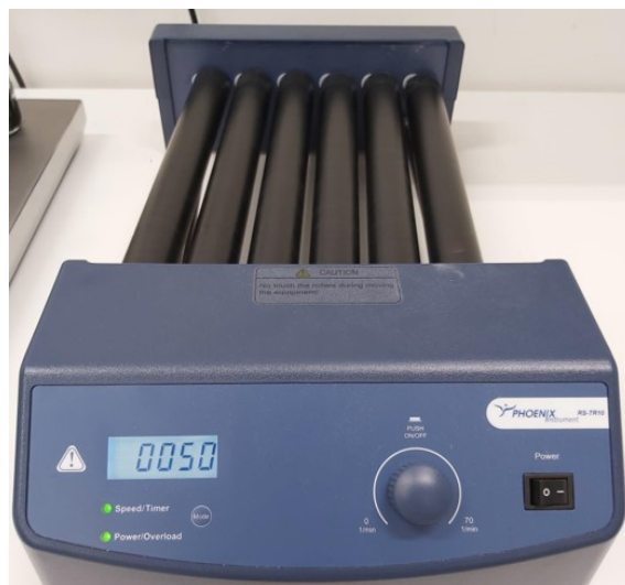
Figure 3.5: Phoenix Instrument RS-TR10 roller shaker used for mixing and dispersing catalytic ink.
