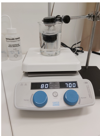
Figure 3.3: Heat treatment set up consisting of a beaker of water with a magnetic stirrer on a hot plate fitted with a temperature probe. The sample is clamped and held suspended in the water.
