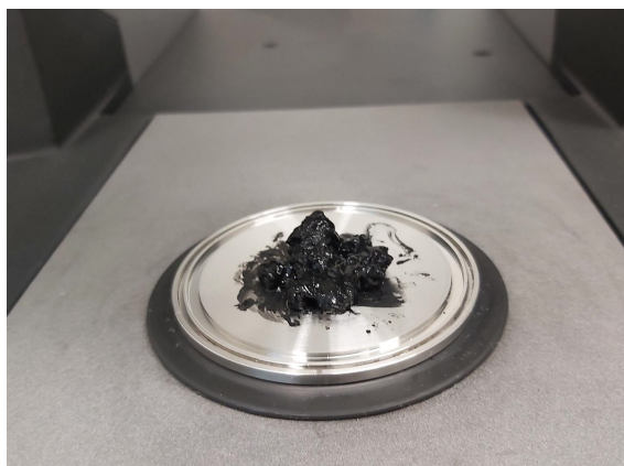
Figure 4.34: Fully solidified tert-butanol and A1 based catalytic ink mixed according to Table 4.5.3.1.
