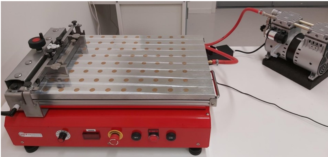
Figure 3.7: MTV CX4 Film applicator with doctor blade used for electrode coatings.
