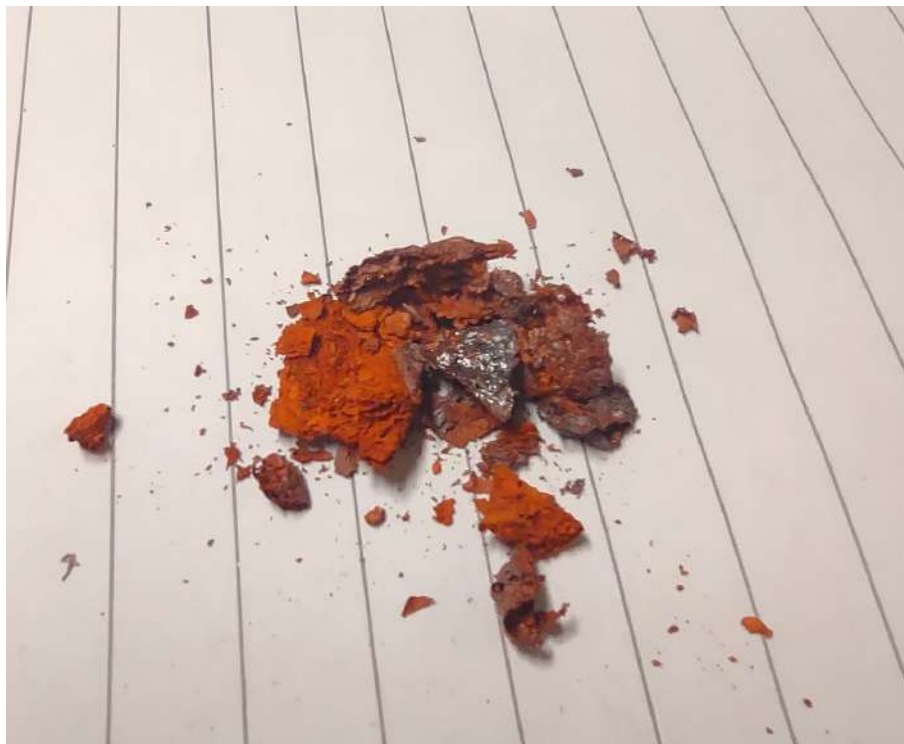
Figure 3.6: Finished material impregnated with iron and cerium. Note the metallic gray piece at the centre, possibly indicating excessive metal loading.
