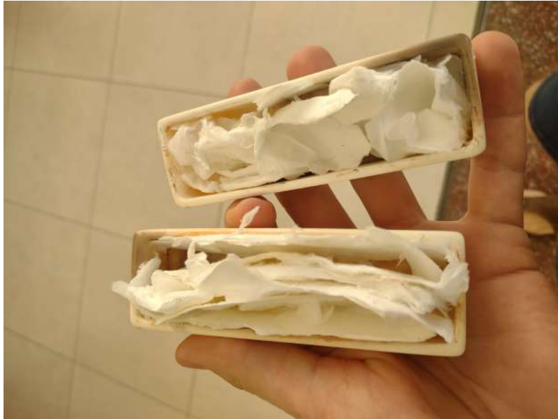
Figure 3.2: Unstabilized fibre sheet loaded into crucibles.
