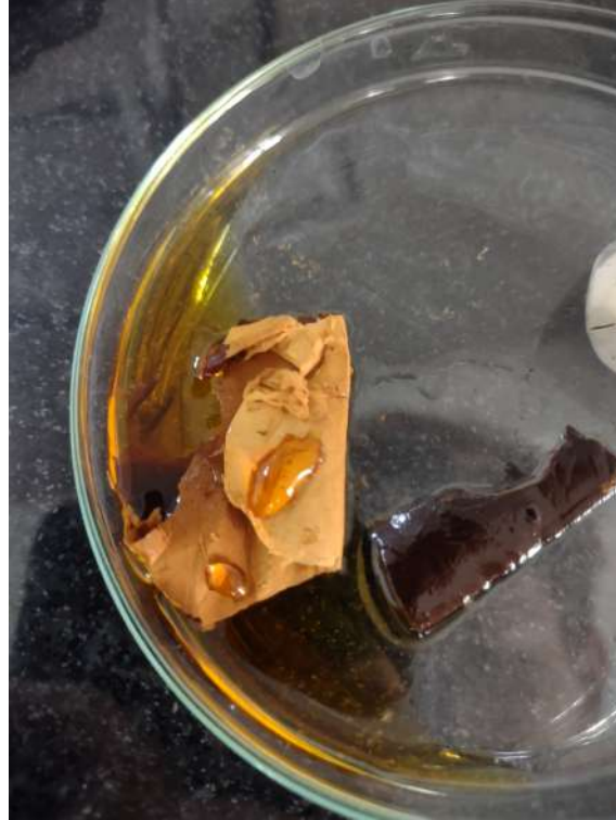
Figure 3.4: Poor wetting can be seen on fibres which have not been completely stabilized to the left. A piece of correctly stabilized fibres can be seen to the right in the dish which readily absorbs the solution.
