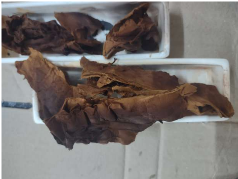
Figure 3.3: Stabilized fibres in crucible. While there is a clear colour gradient which indicates uneven stabilization, pieces within this colour span would reliably absorb the impregnation solution.
