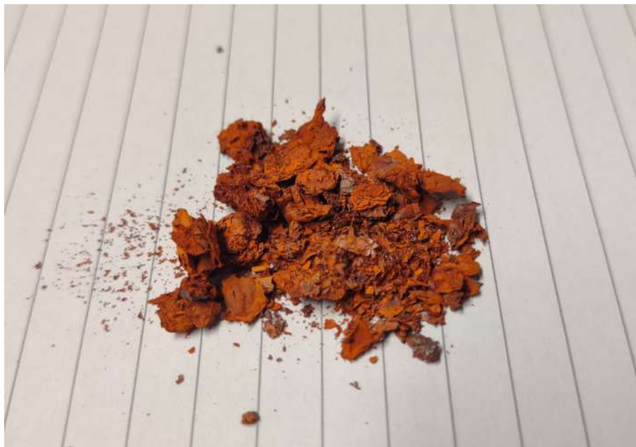
Figure 3.5: Finished material, the sample shown is only impregnated with iron.
