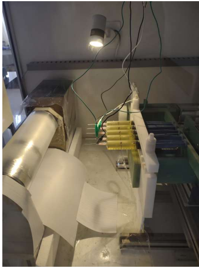
Figure 3.1: Inside setup of the electrospinning machine. Syringe pump with filled syringes can be seen on the right and the collector drum is seen to the left in the image.
