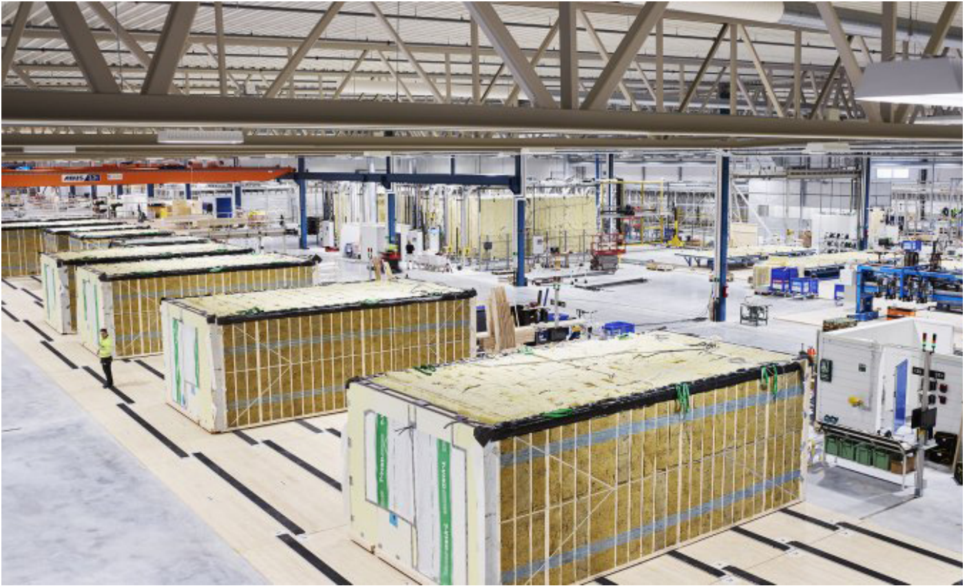
Picture 10. Volume modules in the production line at Lindbäck's factory, source: Lindbäck's Bygg AB
