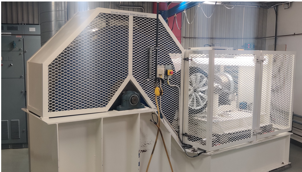
Figure 3.1: ‘Rig-0455’ rolling resistance measurement machine at Volvo Cars
