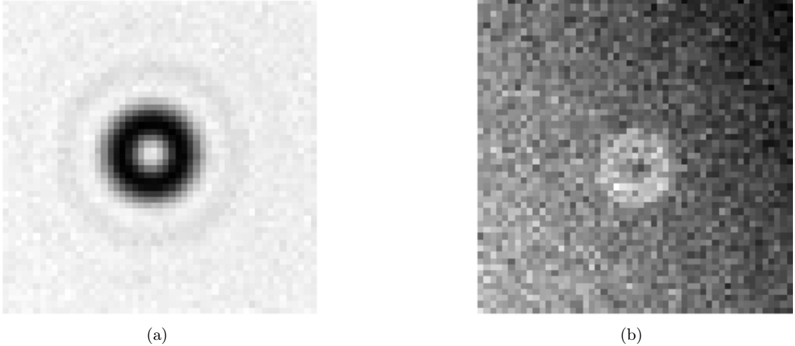
Figure 3.19: Example images sampled from typical training images of DeepTrack. In fig. 3.19a with a SNR of 100 and in fig. 3.19b with a SNR of 10. The task is to locate the center of the particle. The images are 51 \times 51 pixels.
