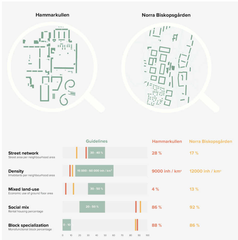
Figure 3.7. Measured data are benchmarked towards guidelines in city planning theory. This analysis creates an evident baseline upon which design decisions for urban development can be made (Forsemalm & Göransson, 2019).
