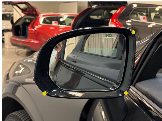
Figure 4.5: Reference markers (three yellow dots) on the left rear mirror.
