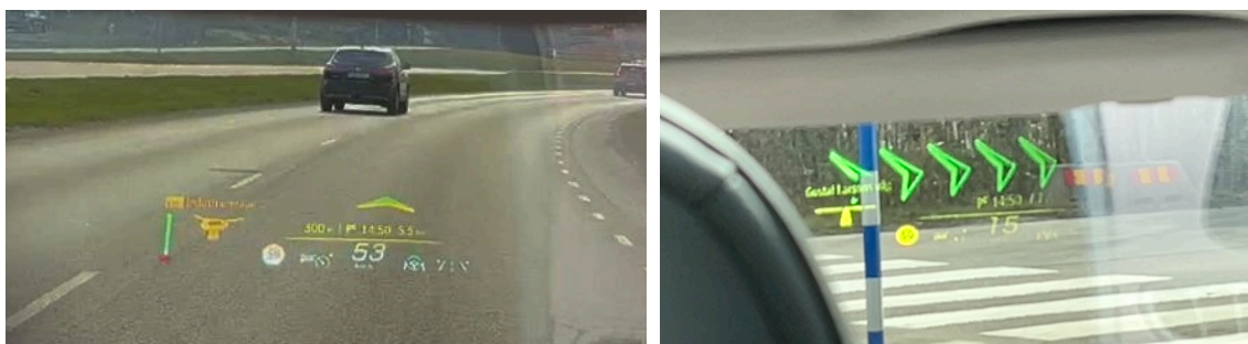
Figure 2.4: AR-HUD in the Mercedes-Benz S-Class, providing a wide FoV and dynamic symbols.
