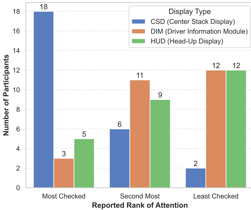
Figure 5.5: Distribution of participant-reported navigation display usage. Participants ranked three display types (CSD, DIM, HUD) according to how often they typically checked the displays for navigation information while driving.
