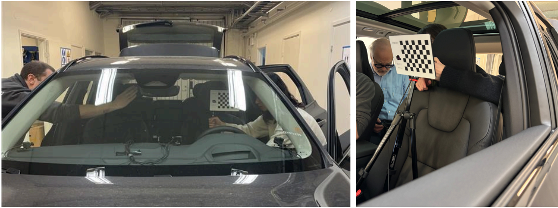
Figure 4.4: The laser chessboard shoots lasers on the reference markers to get the coordinates in relation to the WCS.
