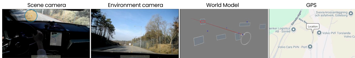
Figure 4.9: Synchronised scene camera, environment camera, world model, and GPS in iMotions.
