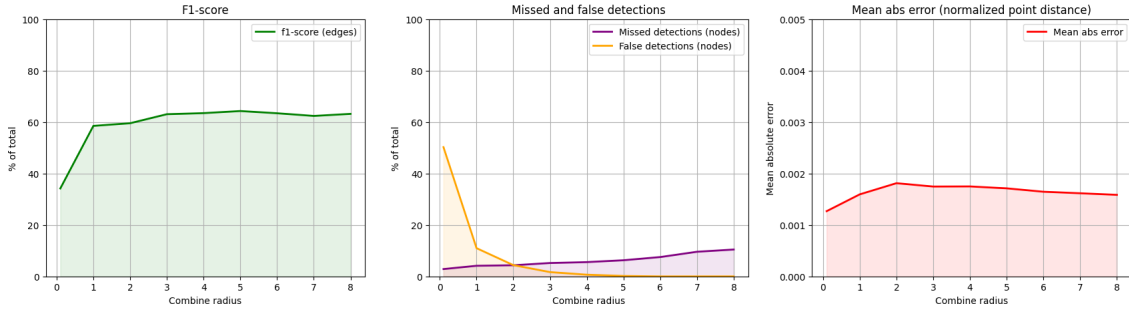
Figure 4.7: F1-score, missed detections, false detections, and mean absolute error between the detection and target for different radii for which detections are combined.
