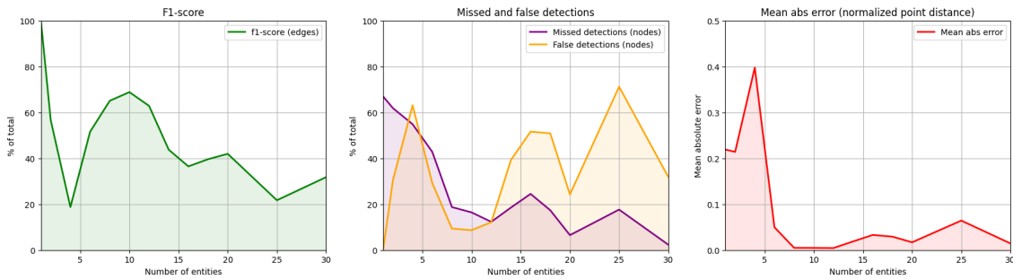
Figure 4.8: F1-score, missed detections, false detections, and mean absolute error between the detection and target for different values of the hyperparameter "number of entities".
