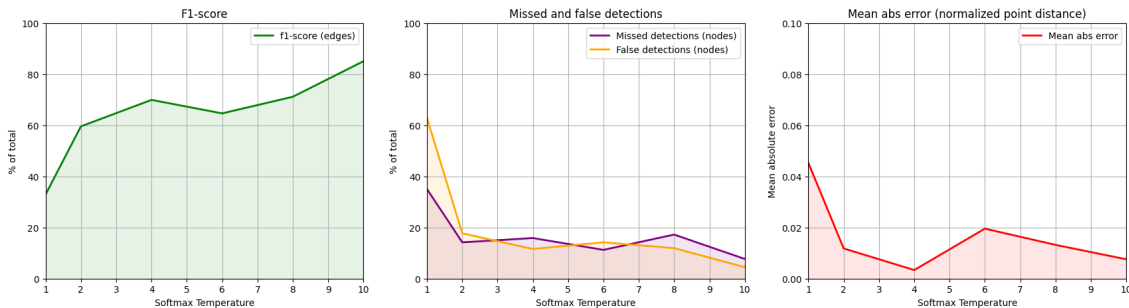
Figure 4.9: F1-score, missed detections, false detections, and mean absolute error between the detection and target for different values of the hyperparameter "softmax temperature".
