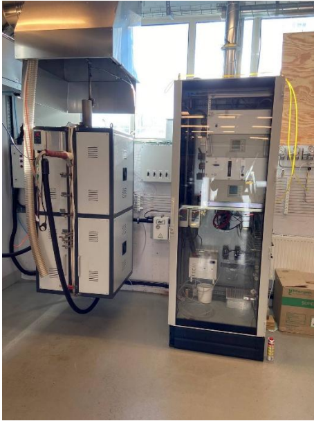
Figure 3.2 : Reactor X inside the furnace with SICK gas analyzer
