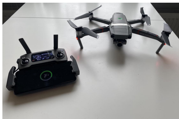
Figure 2.3: The DJI Mavic 2 Enterprise Drone with controller
